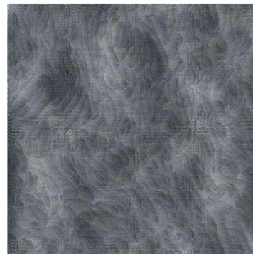
Figure 1: Typical atomic force micrograph ( $10 \times 10 \mu\text{m}^2$  area) of an AlGaN/GaN structure grown for this sample series. The root mean square surface roughness is 0.25 nm.
