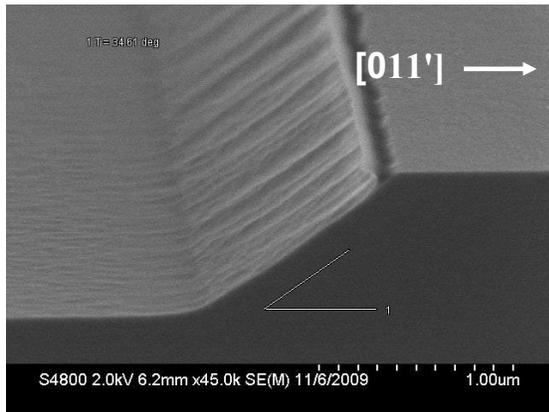
Figure 4: Sample with NH<sub>4</sub>OH based pre-coat treatment and NH<sub>4</sub>OH based pre-etch clean from the DOE.
