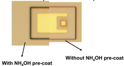
Figure 7: HBTs after the base/collector etch overlayed to show the difference in the mesa top width when a pre-coat treatment is used.
