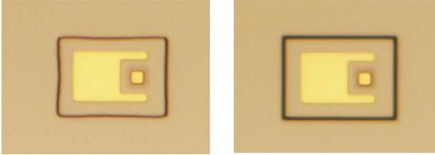
Figure 6: Devices viewed after the base-collector etch with no pre-coat treatment (left) and device with  $\text{NH}_4\text{OH}$  pre-coat treatment (right). The base mesa is designed to be  $22 \times 28.5 \mu\text{m}$ .
