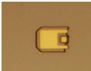
Figure 1: Typical HBT from early lot with severe resist adhesion failure after partial processing.
