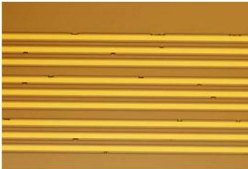
Figure 2: Serpentine structures viewed after the base-collector etch with no pre-coat treatment. These images show a failure mode that is much more localized, but was also remedied by the pre-coat treatment.
