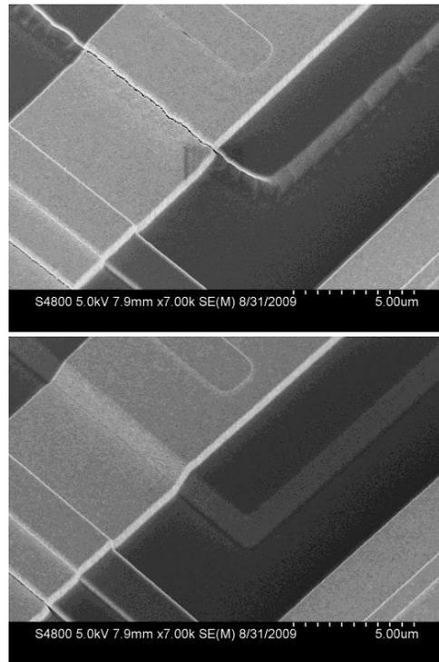
Figure 5: SEM images showing metal discontinuity for the sample with no pre-coat treatment (top) and smooth metal coverage for sample with pre-coat treatment (bottom).
