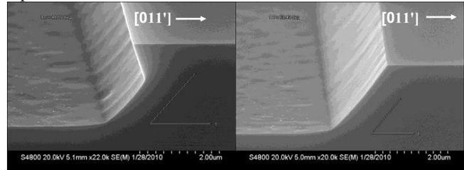
Figure 3: Wet etch profile of (100) GaAs etched without a pre-coat native oxide etch (left) and with the native oxide etch (right) immediately prior to coat. These samples were immersion etched.
