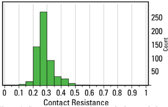
Figure 4: Contact resistance using standard transmission line technique for initial GaNpowIR platform
