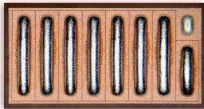
Figure 5: Topside view of a flip chip GaNpowIR device
