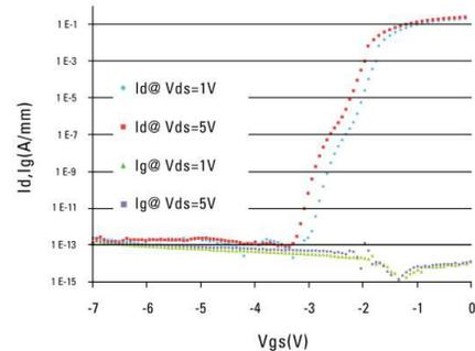
Figure 3: Measured  $I_d$ ,  $I_g$  normalized to gate width ( 850 mm) as a function of  $V_{gs}$  for  $V_d = 1$  and  $5 \text{ V}$ ,  $L_g = 0.3 \mu\text{m}$ .
