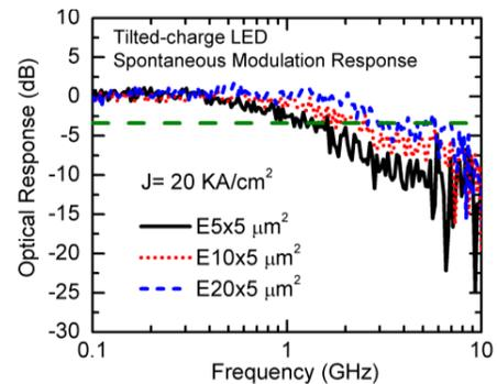
Fig. 4. Response of three different sizes of device under  $J=20 \text{ KA}/\text{cm}^2$  current density.
