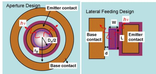
Fig.2 (a) aperture design (b) lateral feeding design
