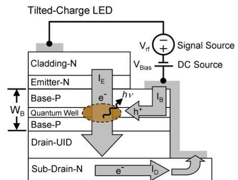
Fig.1 Schematic of tilted-charge LED
