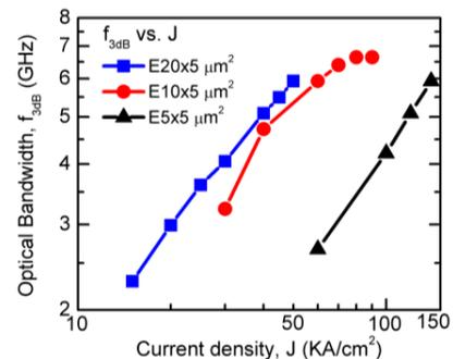
Fig. 5. Optical bandwidth vs. current density for three different devices.
