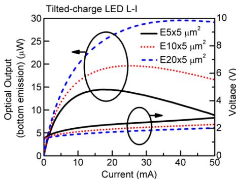
Fig. 3. Electrical and optical characteristics of different emitter mesa of tilted-charge LED.
