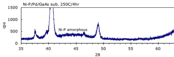
Fig. 6. XRD patterns of Ni-P/Pd/GaAs after annealing for 4 hour at 250°C
