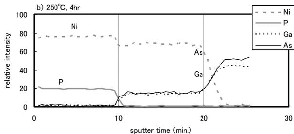
(b) After annealing for 4 hours at 250°C
