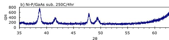
(b) After annealing for 4 hour at 250°C
