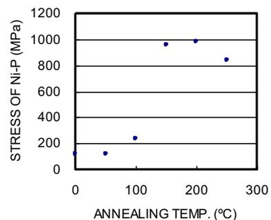
Fig. 1. Annealing temperature dependence of the stress of Ni-P layer
