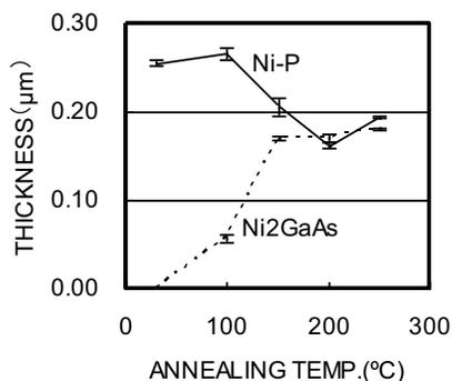
Fig. 3. Annealing temperature dependence of Ni-P, Ni<sub>2</sub>GaAs thickness
