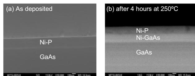
Fig. 2. SEM image of vertical cross section of As-Deposited Ni-P on GaAs and after annealing for 4 hour at 250°C
