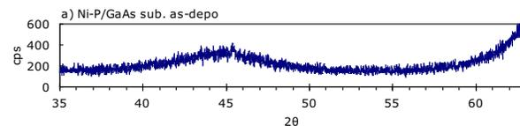
(a) as deposited Ni-P/GaAs
