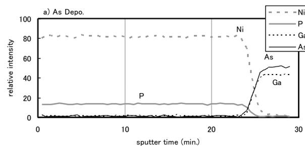
(a) as deposited Ni-P on GaAs
