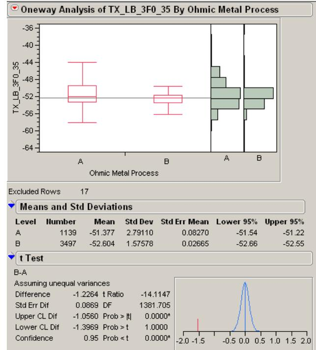
Figure 6 Best Process Condition (B) vs Original Process (A)
