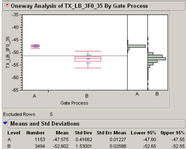
Figure 4 Switch Arm Leakage Current vs Gate Process Condition
