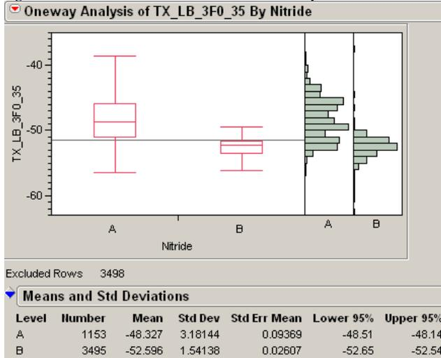
Figure 3 915 MHz Third Harmonic vs Gate Process Conditions
