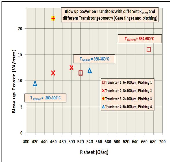
FIGURE 3: Blow up power limits as a function of sheet resistance for different device geometries. Corresponding measured by Raman device temperature at blow up is also given alongside.
