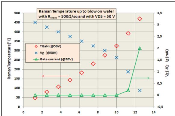
FIGURE 2: T-increase of an 8x400 μm transistor from wafer with  $R_{sheet}$  of 500 Ω/sq as a function of power density, biased with 50V source-drain voltage until blown up. Applied gate voltages and the gate current near the blow up region are given in the figure, too.
