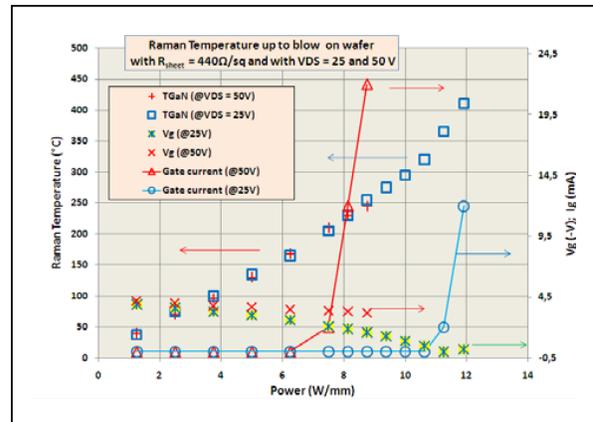
**FIGURE 1: T-increase of a 8x400 μm transistor from wafer with  $R_{sheet}$  of 440 Ω/sq as a function of power density, biased with 25 and 50 V source-drain voltage until blown up. Applied gate voltages and the gate current near the blow up region are given in the figure, too.**
