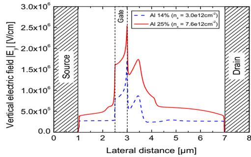
FIGURE 4: Vertical electric field distribution between source and drain in the AlGaN barrier of two AlGaN/GaN epi structures with different Al-content in barrier providing different  $R_{sheet}$  for  $V_{DS} = 50$  V and  $P_{diss} = 2.8$  W/mm.
