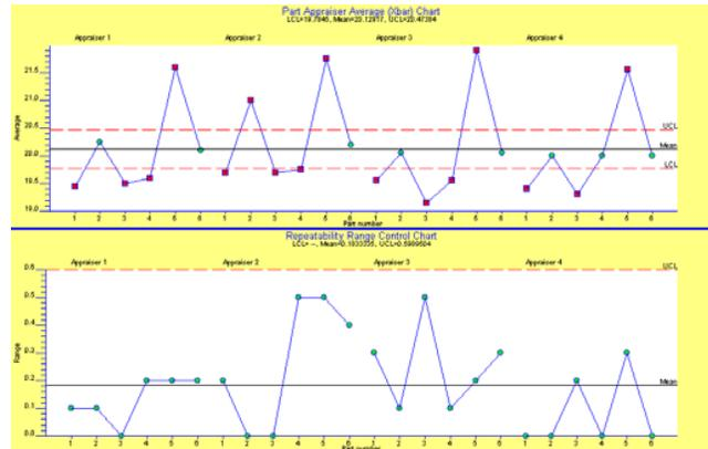
Figure 2: Xbar-R chart for Al composition from XRD Gage Study after increasing X-ray beam intensity.
