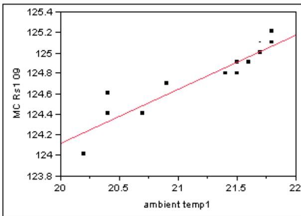
Figure3: Linear fit of correlation between ambient temperature and Rs of GaAs measurement consistency standard.
