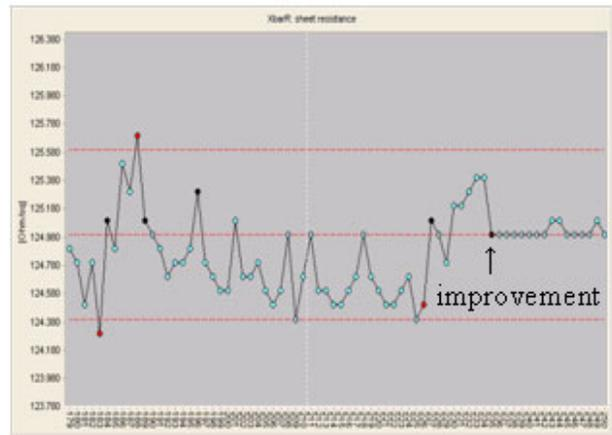
Figure 4: SPC chart of measurement consistency standard Rs before and after including temperature compensation in measurement recipe
