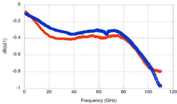
Figure 7: The transition from chip to chip (red curve) adds very little insertion loss to the through measurement (blue curve) between 50 MHz and 110 GHz.
