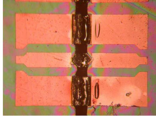
Figure 3: Realization of CPW connection between silicon chips, showing a detail of a coplanar waveguide extending from one chip on the left to a second on the right.
