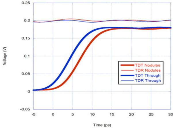
Figure 6: Measured time-domain reflection and transmission data, showing that the reflection is small, and that the delay due to the chip-to-chip transmission adds 2.7 ps to the through measurement.
