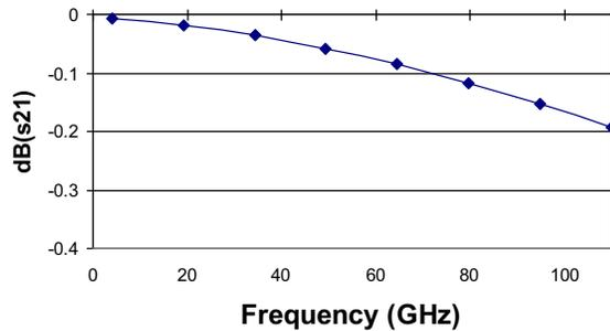
Figure 8: Predicted insertion loss (using Ansoft HFSS) for an optimized nodule line on GaAs, as a function of frequency.
