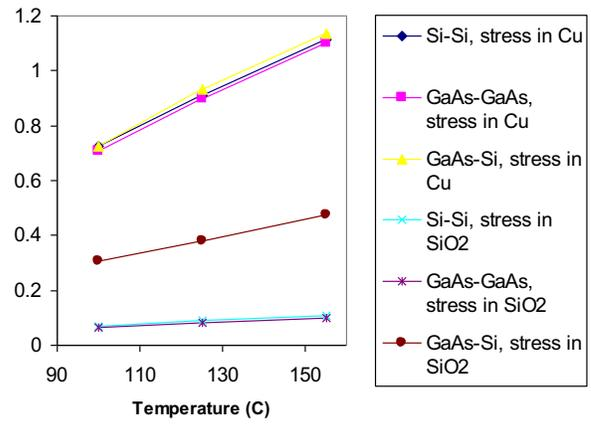
Figure 9: The maximum normalized values of von Mises stress is plotted for each combination of chip connections. The von Mises stress in the copper is normalized to 220 MPa, while the stress in the oxide is normalized to 50 GPa.
