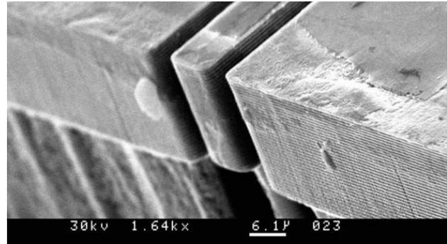
Figure 4: Side view of a 10  $\mu\text{m}$  thick and 20  $\mu\text{m}$  deep copper QP nodule on silicon substrate.
