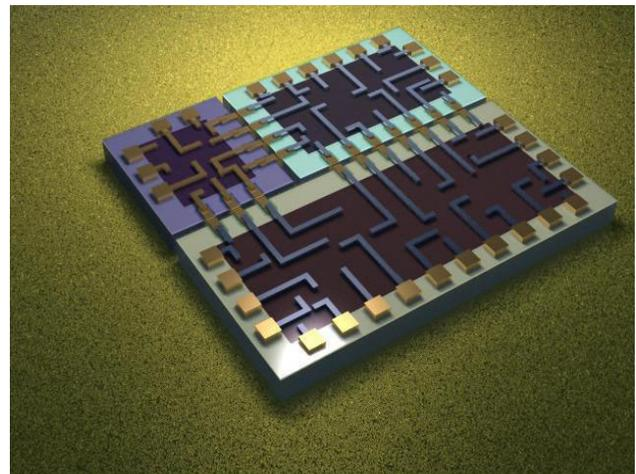
Figure 2: Rendering of a “metachip” –three chips interfaced by high speed QP interconnects.
