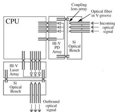
Figure 1: Concept of several technologies interfaced by QP to use the best qualities of each, optimizing performance of the overall system.
