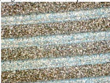
FIGURE 4 PLATE TEXTURE BY MICROGROOVING (FACING) AT 50X
