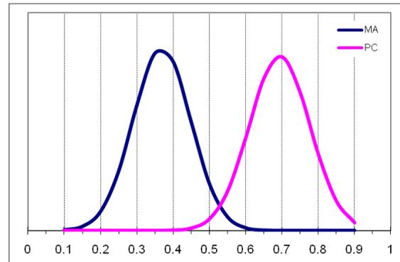
FIGURE 8 CUT RATE COMPARISON FOR LAPPING R-PLANE SAPPHIRE USING 3 $\mu$ m DIAMOND ON HY-CU PLATE, DIAMOND TYPE MA VS. PC.
