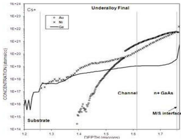
Fig.3. Backside SIMS profiles of 'under-alloyed' sample at the end of fabrication processes
