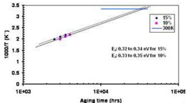
Fig.4. Arrhenius activation energy plots of inverse of absolute temperature vs. failure time
