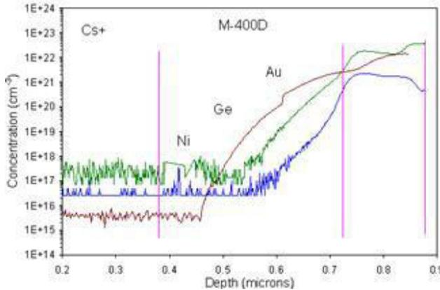
Fig. 2. Backside SIMS profiles of optimally alloyed sample at the end of fabrication processes
