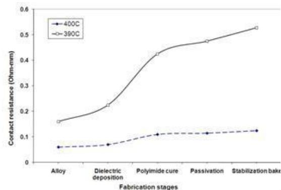
Fig. 1. Drift of  $R_c$  during fabrication stages
