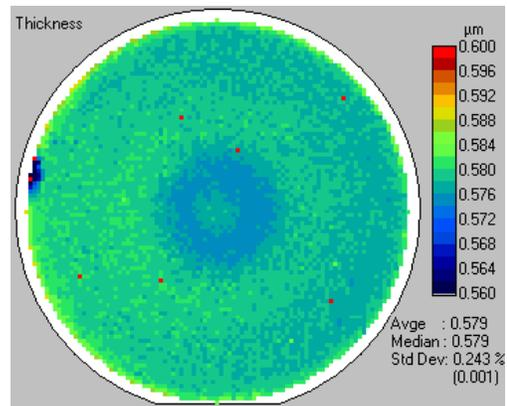
Figure 4: Thickness mapping from a GaN layer, grown on 200 mm sapphire using low temperature nucleation conditions, by post growth white-light interference (Nanometrics rpm VERTEX®). The thickness uniformity, only  $\sigma = 0.24\%$  (with 6 mm edge excl.), indicates the uniformity of the gas phase delivery.
