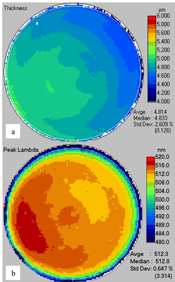
Figure 5: (a) Thickness and (b) PL peak wavelength mappings of a generic LED process run on a 200 mm diameter sapphire substrate.
