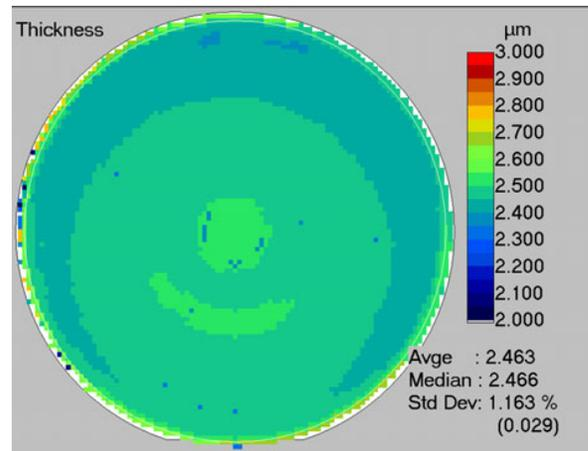
Figure 6: Post growth thickness mapping of an LED structure including 1.3  $\mu\text{m}$  GaN:Si grown on a 200 mm diameter (111) Silicon substrate.
