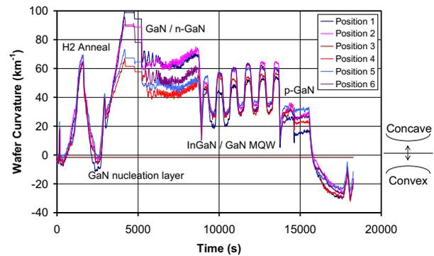
Figure 3. Wafer curvature, measured at 6 positions at 60° intervals around the circumference, during LED growth on 200 mm diameter sapphire.
