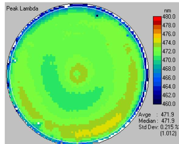
Figure 7: Post growth PL peak wavelength mapping of an MQW grown on a 200 mm diameter (111) Silicon substrate.
