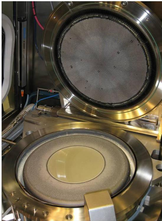
Figure 2: Photo of the Crius® Closed-Coupled-Showerhead MOCVD reactor opened after the growth of an LED structure on 200 mm sapphire.
