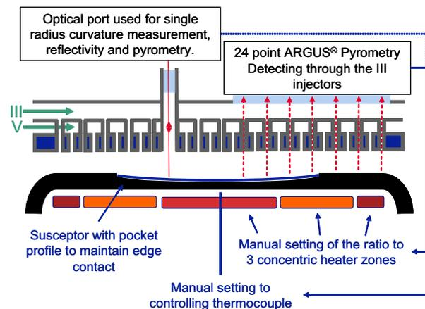
Figure 1: Schematic of the Crius<sup>®</sup> reactor with in-situ monitoring. The 200 mm wafer sits on a susceptor heated by 3 concentric radial heater zones, which are adjusted throughout the process to optimize the temperature profile on the wafer based on in-situ measurements by Argus<sup>®</sup>.
