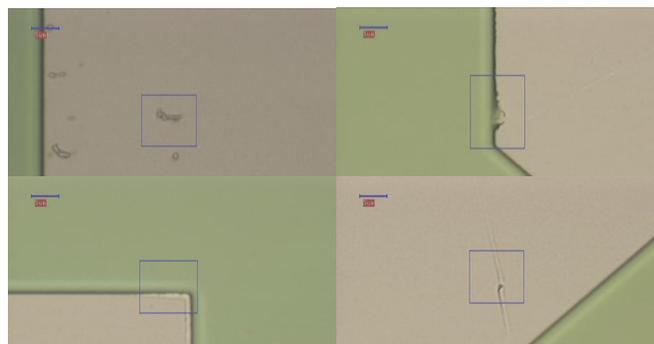
Figure 6: Typical defects found on the bottom electrode, from top left clockwise: lift-off metal residues; edge breaking, scratches, resist residues
