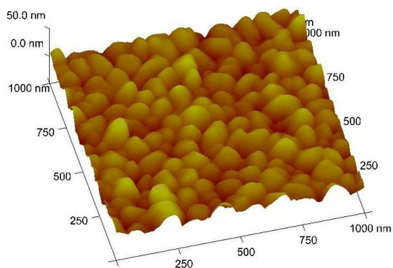
Figure 5: AFM record of the bottom electrode of the MIM structure.
