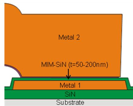
Figure 1: MIM-Structure, as used in this investigation.
