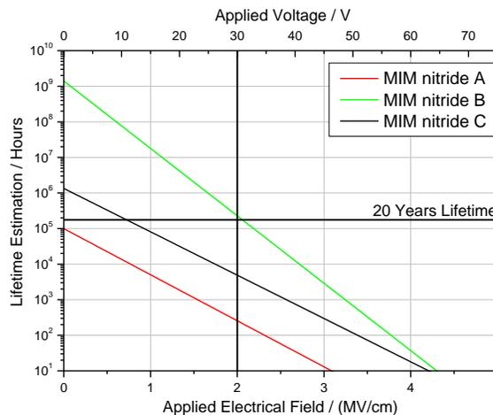
Figure 9: Lifetime estimation for the different nitrides; only MIM nitride B is able to deliver 20 years of lifetime.
