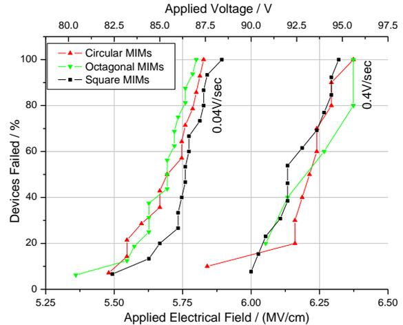
Figure 3: Distribution of failures for different geometries.
