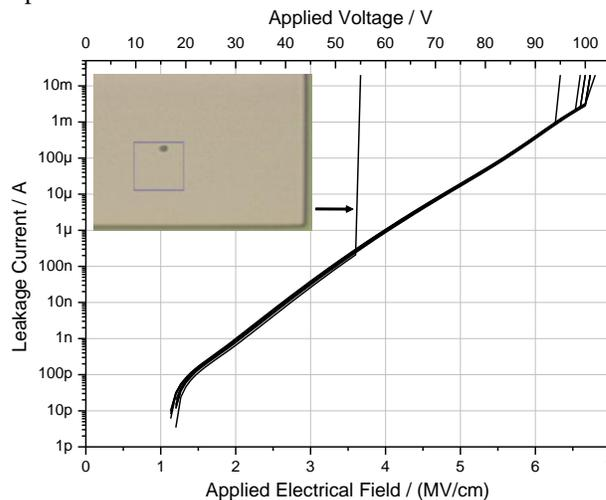
Figure 7: IV-characteristics of  $4 \times 10^{-2} \text{ mm}^2$  big MIMs with homogeneous breakdown; one early failure is visible.
