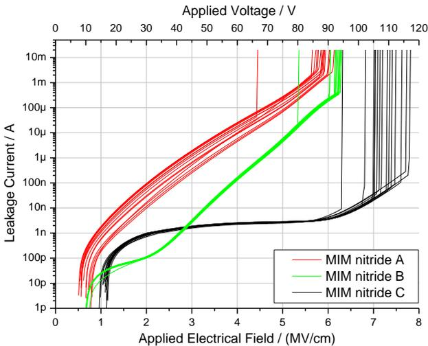
Figure 2: IV-characteristics of the different SiN types.
