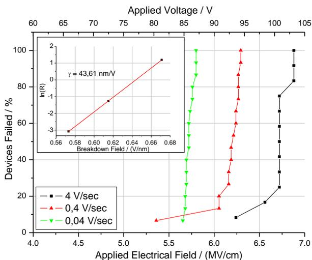
Figure 8: Failure distribution of MIM nitride B for different ramp rates; the inset plot shows the corresponding determination of the acceleration factor.
