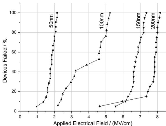
Figure 4: Failure distribution for different nitride thicknesses.
