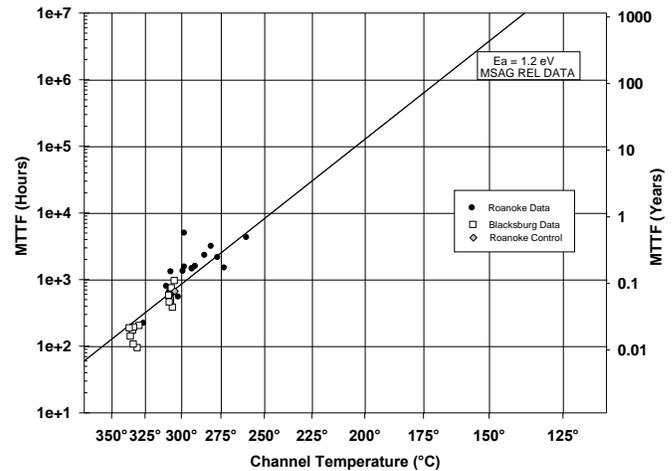
Figure 5. Arrhenius plot of RF-biased accelerated life test results for MSAG FETs. Blacksburg results (□) match results from tests performed in Roanoke on Roanoke-fabricated devices (●).
