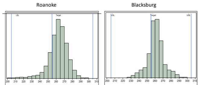
Figure 3. Histograms for BFET Idss comparing Roanoke to Blacksburg. Here, the short-term Cpk for Blacksburg was demonstrated to be slightly better than that for Roanoke.
