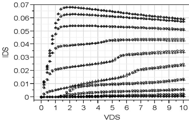
Figure 2. dc IV plots of MSAG 5A FET showing identical behavior Blacksburg (o) vs Roanoke (+). Data was taken at the ohmic-level part of the process at which point FETs are fully functional for dc measurement.
