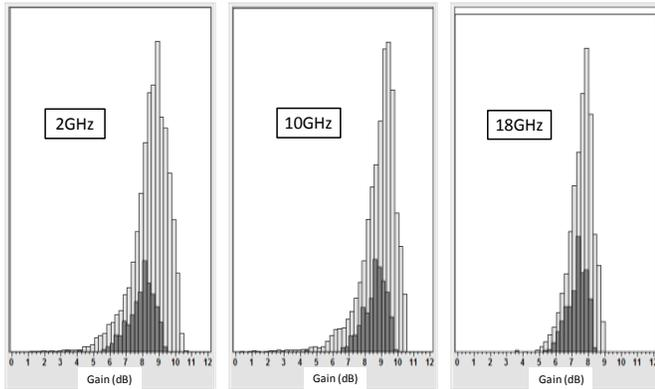
Figure 4. Histogram plots which illustrate the Roanoke (□) vs Blacksburg (■) performance comparison, over frequency, for small signal gain of a Broadband Low Noise Amplifier. Performance-comparison behavior similar to this was obtained for all specified parameters on this circuit as well as the other circuit types tested as part of the OWT circuit performance qualification.
