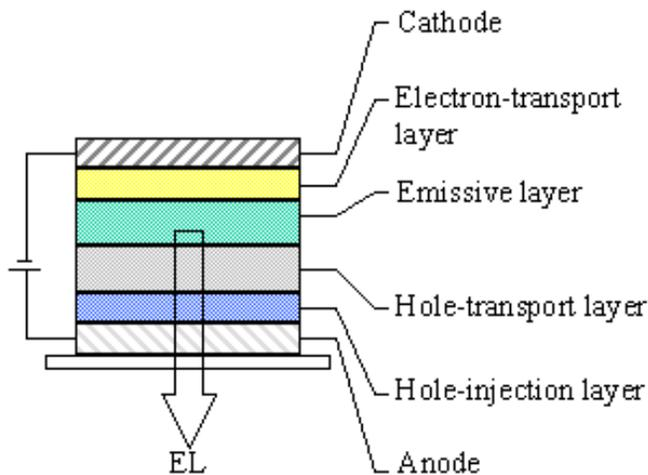
Figure 3: Typical OLED device structure
