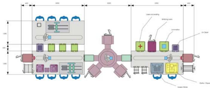
Figure 4: LACE OLED prototyping line
