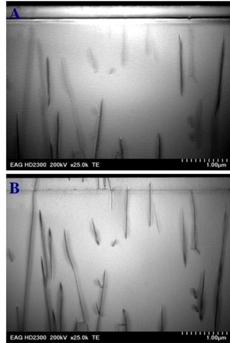
Figure 3: STEM bright field image of dislocations with screw (A-top) and edge (B-bottom) components.
