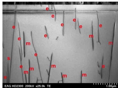
Figure 4: STEM bright field image of dislocations with screw (top) and edge (bottom) components. All dislocations are characterized by their types (e-edge, m-mixed, s-screw).
