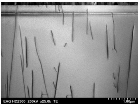
Figure 2: STEM bright field image of dislocations with all components of VTDs.
