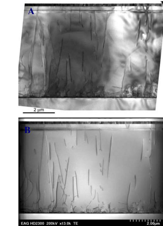
**Figure 1: Comparison of TEM and STEM imaging of VTDs in GaN m-plane. (A) TEM bright field image showing contrast from dislocations as well as thickness fringes, bend contours and Kikuchi diffraction pattern. (B) STEM bright field of the identical sample as in (A) showing simplified and uniform contrast.**
