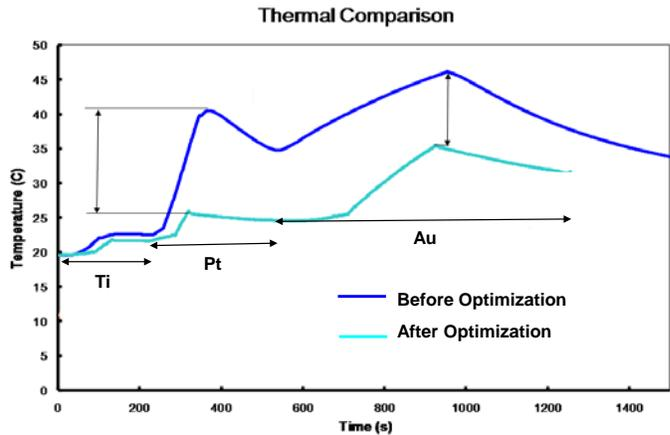
Figure 5. Thermal cycle comparison of ebeam evaporator optimization.
