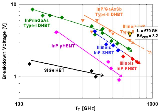
**Figure 1.** Breakdown voltage versus  $f_T$  scaling relationship of the various InP-based HBTs compared to InP pHEMTs and SiGe HBTs.
