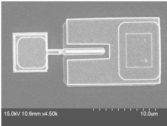
Figure 7. SEM of sub-micron HBT device (top view).
