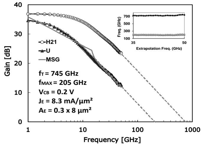
Figure 8. Measured RF data with extrapolations to  $f_T = 745$  GHz and  $f_{\text{MAX}} = 205$  GHz for device with  $A_E = 0.3 \times 8 \mu\text{m}^2$  on 20nm base, 60nm collector structure biased at  $-37^\circ\text{C}$ .
