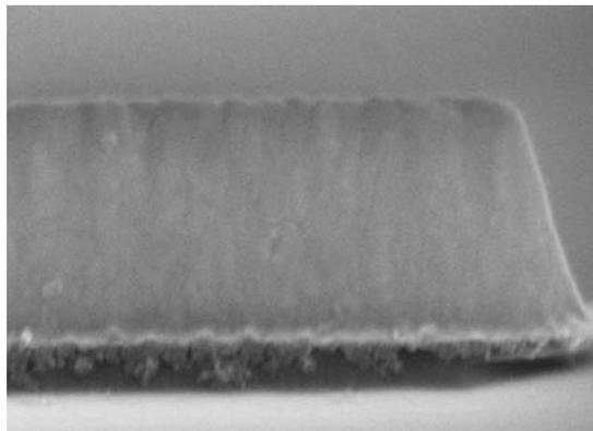
Figure 4. Emitter “wing” collapse after emitter mesa etch. The folded metal filament can cause emitter to base short.
