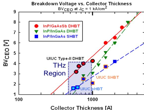
**Figure 2.** Reported off-state breakdown voltage versus collector layer thickness for InP SHBT/PHBT, type-I DHBT, and type-II DHBT. THz cutoff frequency devices will have collector layer thicknesses from 500 to 1000 Å.
