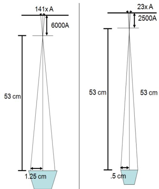
Figure 6. The crucible size and imaging resist thickness determine the emitter wing size by solid angle lines illustration.
