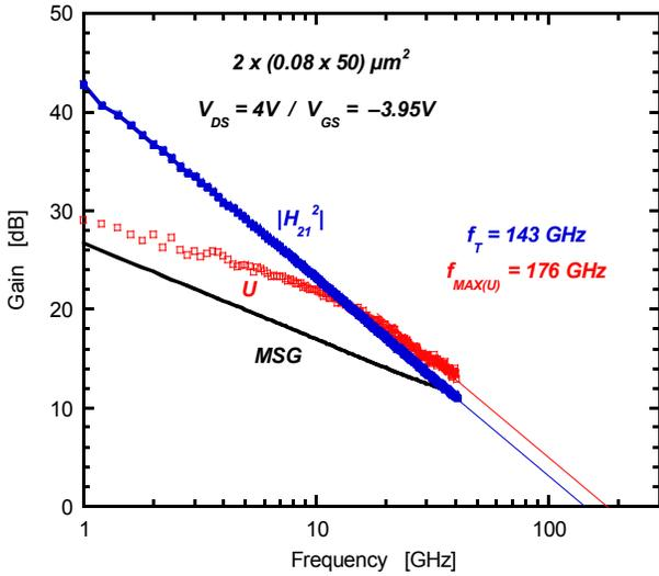
Figure 3. Microwave response for  $2 \times (0.08 \times 50) \mu\text{m}^2$  HEMT on HR-silicon. Extrapolation at  $-20$  dB/dec yields  $f_T = 143$  GHz and  $f_{\text{MAX}(U)} = 176$  GHz at  $V_{\text{DS}} = 4$  V and  $V_{\text{GS}} = -3.95$  V [9].
