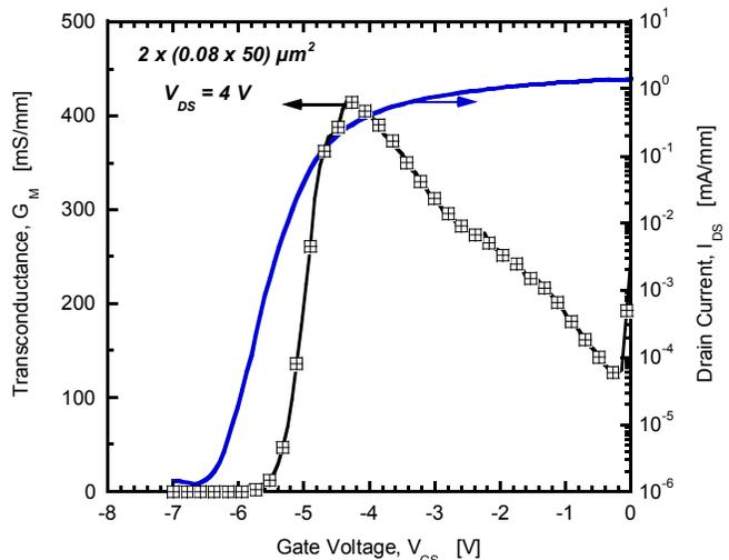
Figure 2. Transconductance and *I*<sub>D</sub>-*V*<sub>GS</sub> transfer characteristic for 2 × (0.08 × 50) μm<sup>2</sup> HEMT measured at *V*<sub>DS</sub> = 4 V. The *I*<sub>ON</sub>/*I*<sub>OFF</sub> ratio is > 10<sup>6</sup> [9].
