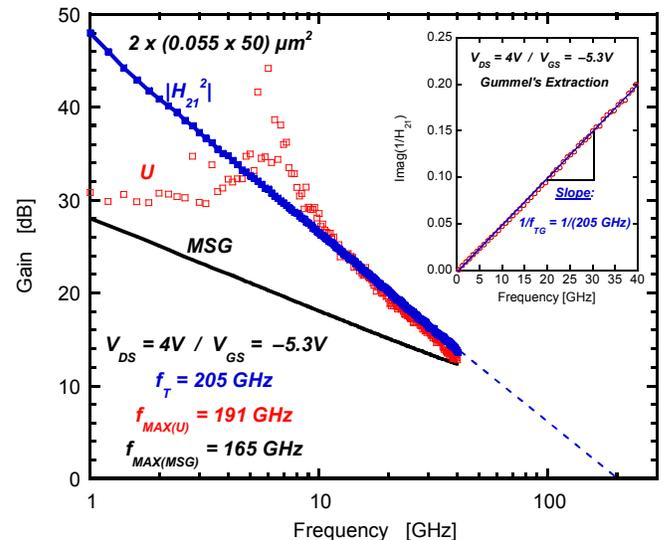
Figure 5. Small-signal frequency response measured at  $V_{\text{DS}} = 4$  V and  $V_{\text{GS}} = -5.3$  V [10]. Inset:  $f_T$  extraction using Gummel's method [11].
