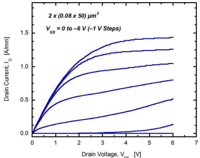
Figure 1. Drain characteristics of 2 × (0.08 × 50) μm<sup>2</sup> devices measured for *V*<sub>GS</sub> = 0 to -6 V, in steps of -1 V [9].
