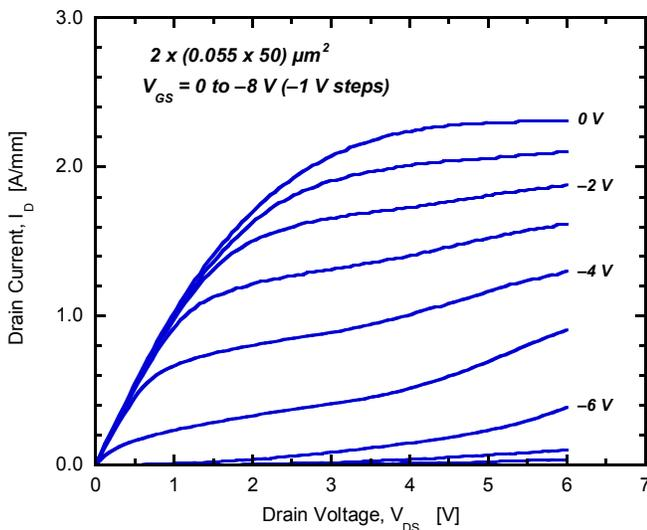
Figure 4. Drain characteristics of  $2 \times (0.055 \times 50) \mu\text{m}^2$  HEMT measured from  $V_{\text{GS}} = 0$  to  $-8$  V, in steps of  $-1$  V [10].
