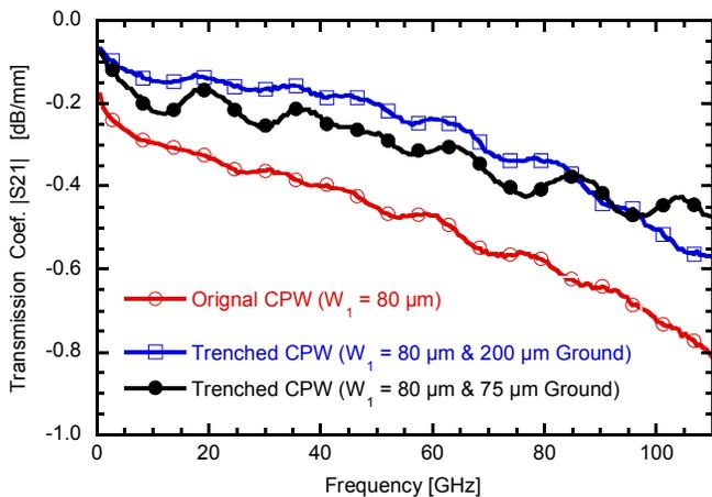
Figure 5. Measured transmission coefficient of CPW with an 80  $\mu\text{m}$  wide center conductor, showing the original design, and two trenched designs with 200 and 75  $\mu\text{m}$  ground plane widths. The trench etch depth was approximately 10  $\mu\text{m}$ .
