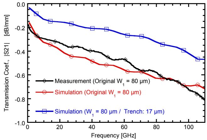
Figure 3. Comparison between measurement and simulation of the CPW with  $80 \mu\text{m}$  center conductor and simulation of an optimized structure with trenches between the metallization.
