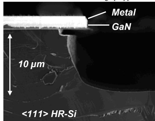
Figure 4. Scanning electron micrograph (SEM) image of cleaved CPW transmission line showing the trench between the center conductor and the ground planes. The trench depth was approximately  $10 \mu\text{m}$ .
