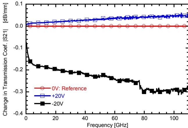
Figure 2. Bias dependence of change in transmission coefficient  $|S_{21}|$  with applied potential between the metallization and wafer prober chuck for the low-loss structure with the  $80 \mu\text{m}$  wide centre conductor.
