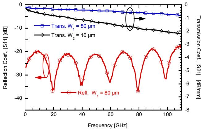
Figure 1. Reflection and transmission coefficients for 3-mm long CPWs with  $W_1 = 80 \mu\text{m}$  and  $W_2 = 10 \mu\text{m}$  center conductor widths. The attenuation at 110 GHz is  $\sim 0.8 \text{ dB/mm}$  for the wide line and  $2.2 \text{ dB/mm}$  for the narrow line. The characteristic impedance of  $W_1 \sim 50 \Omega$  over the full frequency range of interest, as evidenced by  $|S_{11}| \approx -20 \text{ dB}$ .
