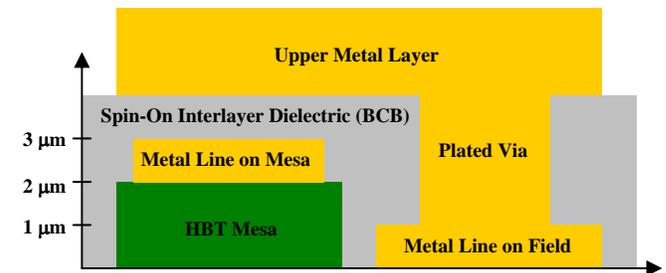
Figure 1. Schematic depiction of power HBT process, showing a HBT mesa of two micron height a one-micron-high metal line over field and over the mesa. (Note that the two micron mesa height includes the effective height of other on-mesa features such as emitter mesa or emitter or base contact metals.)
