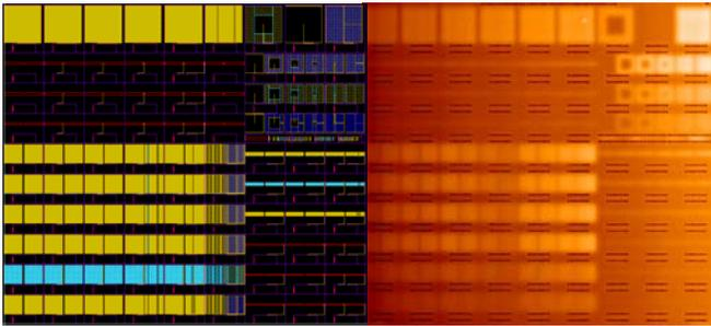
Figure 3. Density characterization reticle field layout shown side-by-side with corresponding measured optical height map after BCB deposition. Brighter regions in image at right indicate taller features after inter-level-dielectric deposition.
