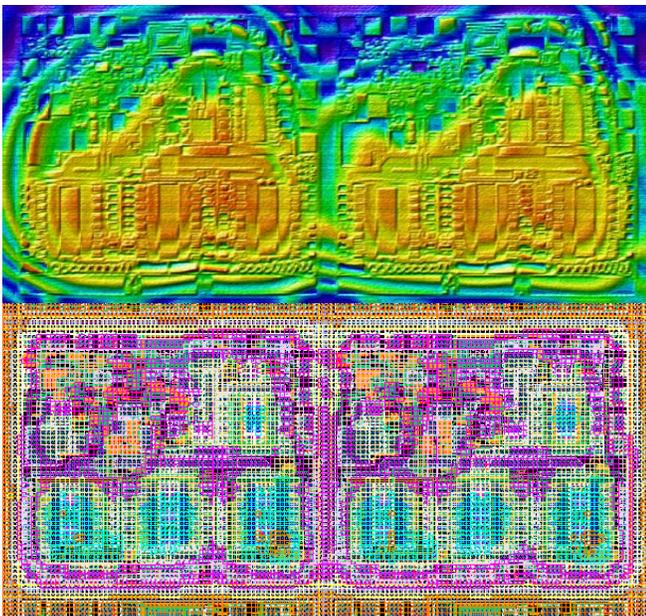
Figure 6. Comparison of optically-measured planarized surface height with design-rule-checker weighted density computation.
