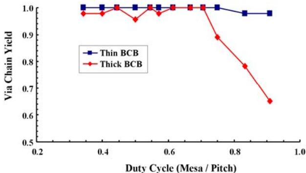
Figure 4. Electrical test results from density characterization maskset showing decreasing via chain yield versus increasing density for a thick BCB split, with no significant yield loss for a split with thinner BCB. The drawn via dimension for the test structures shown is 2.6 microns, and the structure area is 1mm x 1mm, with density features composed of base mesas covered by metal.
