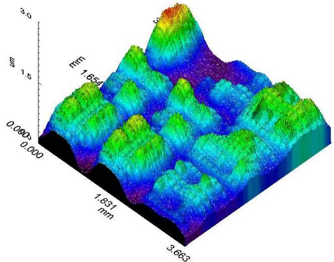
Figure 2. Three-dimensional representation of optically measured surface height profile after BCB planarization of a field from a process development reticle set including many different RF integrated circuit designs.
