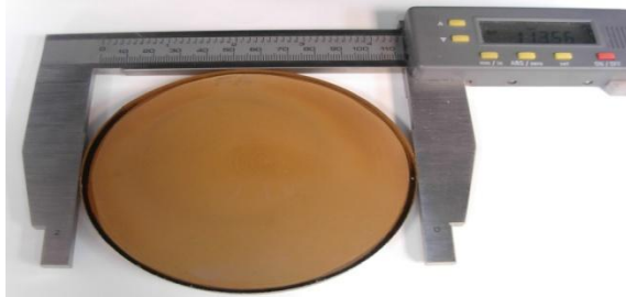
Figure 1 As-grown 113.6 mm 6H SI SiC boule.
