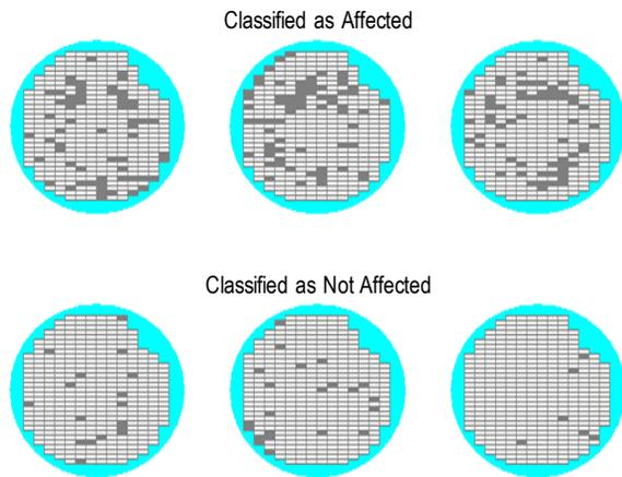
Figure 2. Examples of the sample test bin map signature for affected wafers (top 3 maps) and unaffected wafers (bottom 3 maps). Gray boxes are failing dice; white boxes are passing dice.
