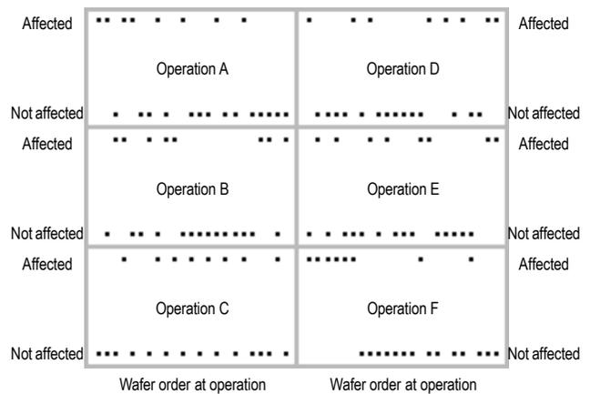
Figure 3. A set of plots showing the presence of the bin map signature vs. wafer order at six different operations on a lot during the late 2004 to early 2005 time frame. Data actually exists for many more operations. Operation C shows a nearly perfect alternating pattern (note that there is a blank space due to a missing wafer). The other operations show much more random dependences.
