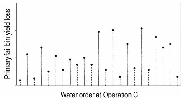
Figure 4. Yield loss from the primary fail bin vs. wafer order at operation C for the same lot as shown in Figure 3. Note that yield loss is in an alternating pattern.
