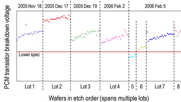
Figure 6. PCM breakdown voltage vs. wafer etch order on multiple lots. Each point shows PCM wafer median. Solid horizontal line indicates spec limit; lot 5 was totally scrapped after failing this limit and triggered this investigation. Note trend of increasing magnitude as more wafers are processed. Four lots were processed consecutively on February 5, 2006, and the trend continues through all 4 lots.
