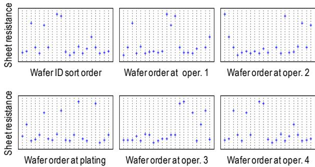
Figure 1. A set of plots showing the median plated metal sheet resistance vs. wafer ID number and wafer order at five operations around and including the plating operation. The plating operation shows a perfect pattern where every fourth wafer has high resistance (note that there is a blank space due to a missing wafer). The other operations show more random dependences.
