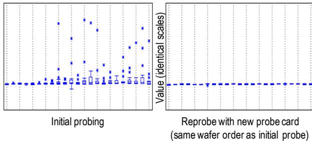
Figure 5. The value of a key electrical parameter vs. wafer order at probing on a single lot, shown as a box plot with points outside the outer fences plotted. The vertical scale is identical between the two plots. The left plot is the initial data; the right plot is reprobe data after the probe card was changed.
