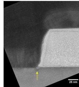
Figure 5: Failure analysis on X-band test structure after RF stress showing etch pit formation
