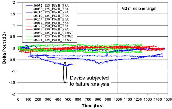
Figure 2: Relative change in RF output power during accelerated RF life test for L-band test structure
