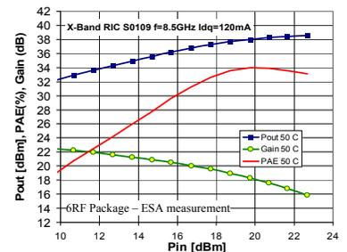
Figure 1: RF performance for L, X-band validation structures
