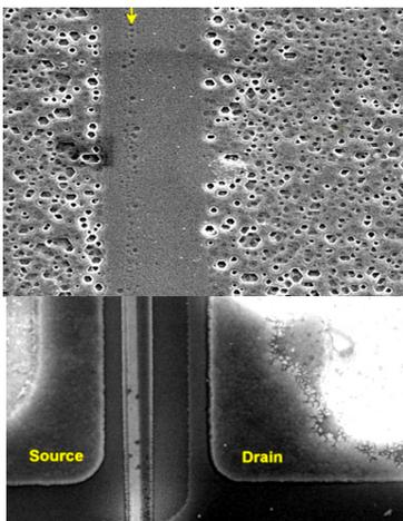
Figure 3: L-band device plan view overlay of gate delayering after RF stress testing
