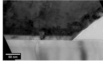
Figure 4: L-band TEM device cross section
