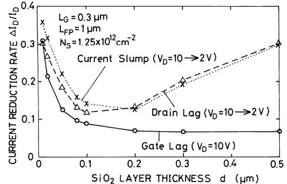
Fig.5. Current reduction rate  $\Delta I_D/I_D$  due to current slump, drain lag or gate lag for GaAs MESFETs, with  $\text{SiO}_2$  layer thickness  $d$  as a parameter.  $L_{FP} = 1 \text{ μm}$ .
