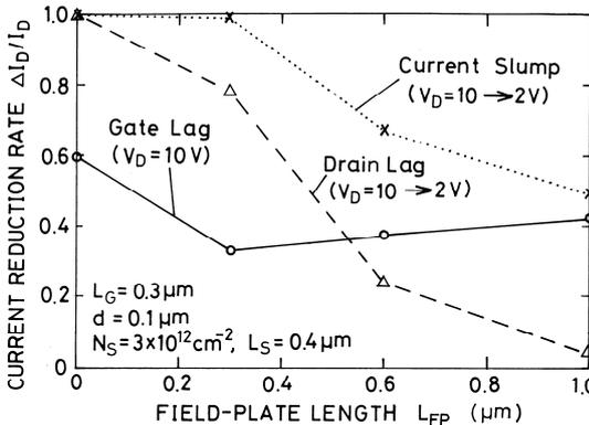
Fig.6. Current reduction rate  $\Delta I_D/I_D$  due to current slump, drain lag or gate lag for GaAs MESFETs, with field plate length  $L_{FP}$  as a parameter.  $d = 0.1 \text{ μm}$ .  $N_S = 3 \times 10^{12} \text{ cm}^{-2}$  and the surface-state length is  $0.4 \text{ μm}$ .
