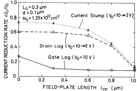
Fig.4. Current reduction rate  $\Delta I_D/I_D$  due to current slump, drain lag or gate lag for GaAs MESFETs, with field plate length  $L_{FP}$  as a parameter.  $d = 0.1 \text{ μm}$ .
