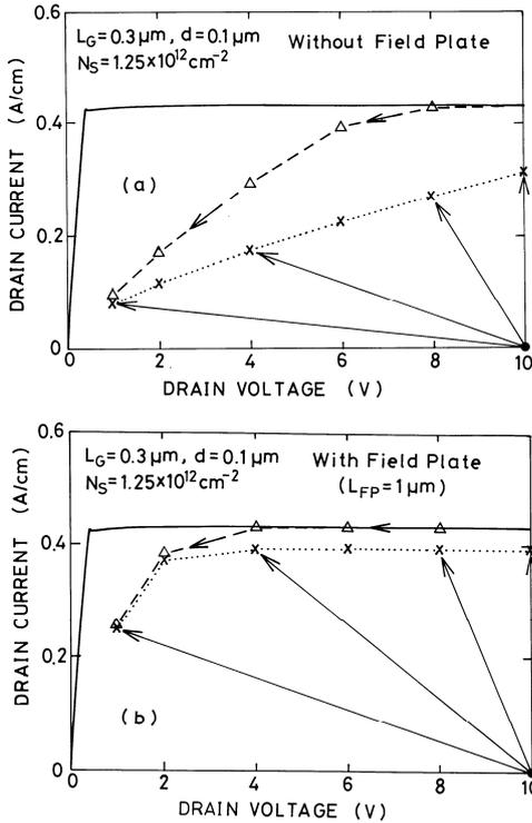
Fig.3. Steady-state  $I-V$  curves ( $V_G = 0 \text{ V}$ ; solid lines) and quasi-pulsed  $I-V$  curves ( $\Delta$ ,  $x$ ) of GaAs MESFETs. (a) Without field plate, (b) with field plate ( $L_{FP} = 1 \text{ μm}$ ). ( $\Delta$ ): Only  $V_D$  is changed from 10 V ( $t = 10^{-8} \text{ s}$ ), ( $x$ ):  $V_D$  is lowered from 10 V and  $V_G$  is switched on from  $V_{th}$  to 0 V ( $t = 10^{-8} \text{ s}$ ).
