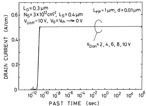
Fig.7. Calculated turn-on characteristics for  $L_{FP} = 1 \text{ μm}$  and  $d = 0.01 \text{ μm}$  when  $V_D$  is lowered abruptly from 10 V to  $V_{Don}$  and  $V_G$  is changed from  $V_{th}$  to 0 V.  $N_S = 3 \times 10^{12} \text{ cm}^{-2}$  and the surface-state length is  $0.4 \text{ μm}$ .
