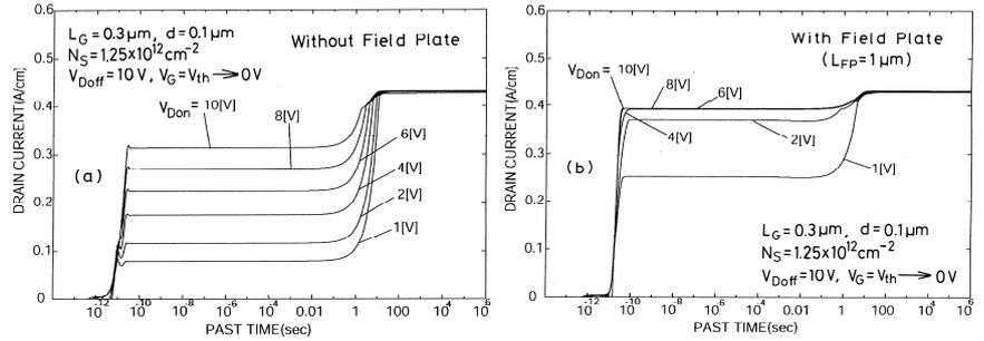
Fig.2. Calculated turn-on characteristics of GaAs MESFETs when  $V_D$  is lowered abruptly from 10 V to  $V_{Don}$  and  $V_G$  is changed from threshold  $V_{th}$  to 0 V.  $N_S = 1.25 \times 10^{12} \text{ cm}^{-2}$ .  $d = 0.1 \text{ μm}$ . (a) Without field plate, (b) with field plate ( $L_{FP} = 1 \text{ μm}$ ).
