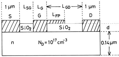
Fig.1 Device structure analyzed here.
