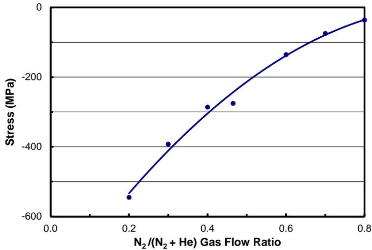
**Figure 1.** Stress control of high rate PECVD  $\text{SiN}_x$  by the He dilution technique. The films were deposited at  $1200 \text{ \AA}/\text{min}$  at a temperature of  $200^\circ\text{C}$ .
