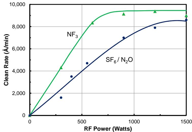
**Figure 2.** Comparison of plasma clean rates *versus* RF power for plasma chemistries of  $\text{SF}_6/\text{N}_2\text{O}$  and  $\text{NF}_3$ .
