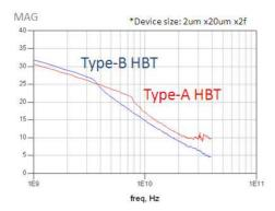
Fig. 2 The comparison results of Maximum Available Gain (MAG) between Type-A and Type-B HBTs. Type-B HBTs show higher MAG than Type-A HBTs for handset application.
