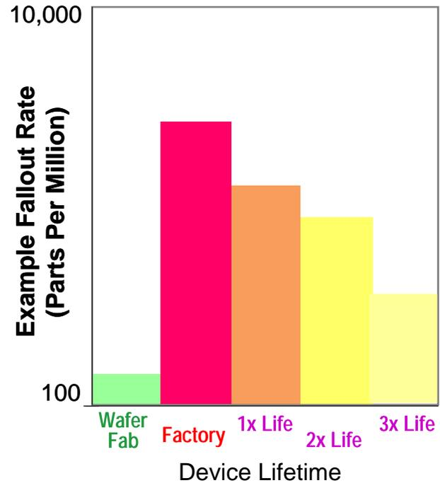
Figure 3. Customer fallout risk assessment based upon multiple accelerated stress tests of 30,000 sample devices from a known maverick lot.
