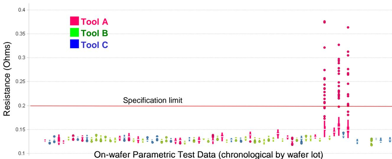
Figure 1. Initial detection of a manufacturing anomaly.
