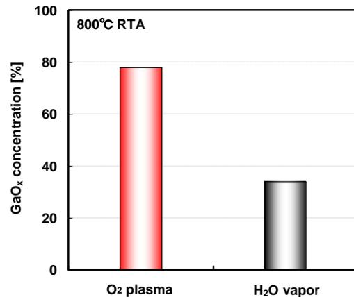
Fig. 7 Comparison of GaO<sub>x</sub> concentration between O<sub>2</sub> plasma and H<sub>2</sub>O vapor-Al<sub>2</sub>O<sub>3</sub>. 800°C RTA was applied in this figure case.
