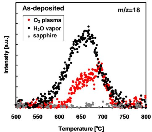
**Fig. 4**  $H_2O$  thermal desorption spectrum of as-deposited  $H_2O$  vapor and  $O_2$  plasma- $Al_2O_3$  measured by TDS.
