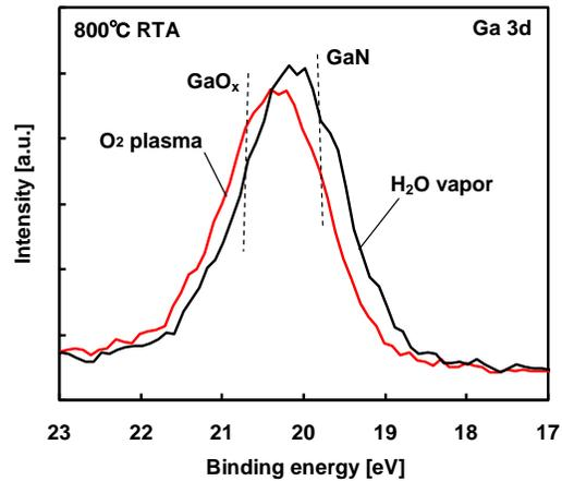
Fig. 6 Ga 3d spectrum at GaN/Al<sub>2</sub>O<sub>3</sub> interface for H<sub>2</sub>O vapor and O<sub>2</sub> plasma-Al<sub>2</sub>O<sub>3</sub> measured by XPS. 800°C RTA was applied in this figure case.
