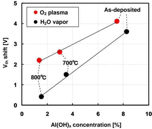
Fig. 5 Al(OH)<sub>x</sub> concentration dependence on V<sub>th</sub> shift for H<sub>2</sub>O vapor and O<sub>2</sub> plasma-Al<sub>2</sub>O<sub>3</sub>. RTA temperature was varied.
