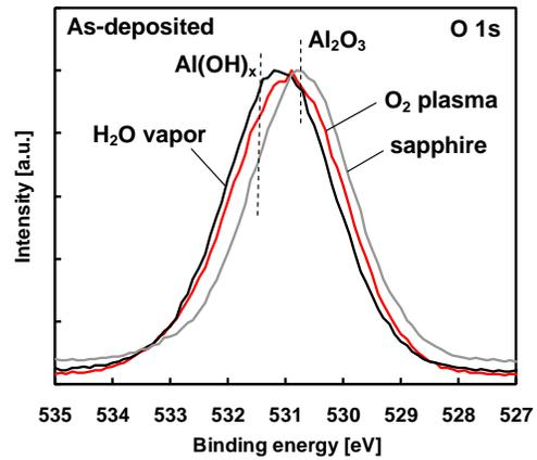
**Fig. 3** O 1s spectrum of as-deposited  $H_2O$  vapor and  $O_2$  plasma- $Al_2O_3$  measured by XPS.
