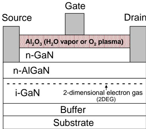
**Fig. 1** Schematic cross-sectional view of normally-on type AlGaIn/GaN MIS-HEMTs structure used in this work.
