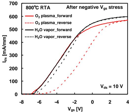
**Fig. 9**  $I_{ds}$ - $V_{gs}$  curves after negative  $V_{gs}$  stress under halogen lamp irradiation for AlGaIn/GaN normally-on type MIS-HEMTs using  $H_2O$  vapor and  $O_2$  plasma- $Al_2O_3$  for gate insulator films.  $800^\circ C$  RTA was applied in this figure case.
