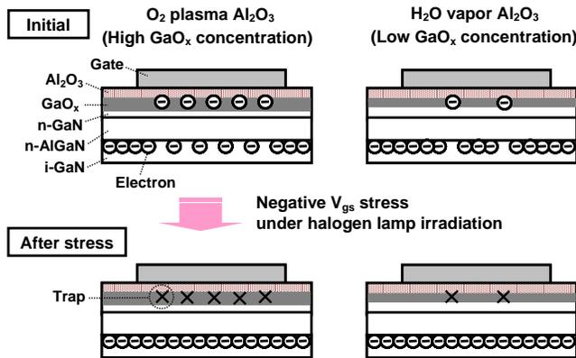
**Fig. 10** Schematic cross-sectional view of the proposed mechanism for the phenomena during negative  $V_{gs}$  stress under halogen lamp irradiation for AlGaIn/GaN normally-on type MIS-HEMTs using  $H_2O$  vapor and  $O_2$  plasma- $Al_2O_3$  for the gate insulator films.
