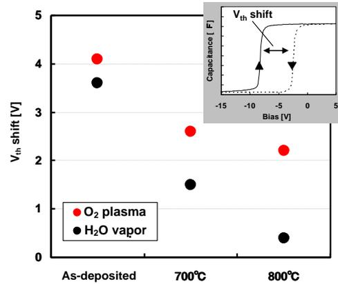
**Fig. 2** Variation in  $V_{th}$  shift with oxidant source and RTA temperature. Upper right inset shows the C-V profile to estimate  $V_{th}$  shift.
