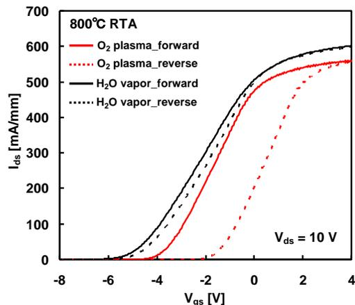
Fig. 8 I<sub>ds</sub>-V<sub>gs</sub> curves for AlGaIn/GaN normally-on type MIS-HEMTs using H<sub>2</sub>O vapor and O<sub>2</sub> plasma-Al<sub>2</sub>O<sub>3</sub> for gate insulator films. 800°C RTA was applied in this figure case.
