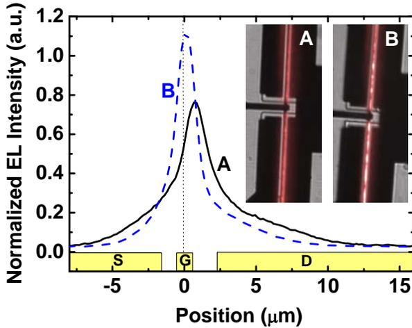
FIGURE 2. ELECTROLUMINESCENCE (EL) PROFILE IN THE SOURCE-DRAIN GAP FOR DEVICE A (SOLID LINE) AND DEVICE B (DASHED LINE), OPERATED AT  $V_{GS} = 0$  V AND  $V_{DS} = 20$  V, MEASURED THROUGH THE BACK OF THE DEVICES, I.E., THROUGH THE SUBSTRATE, TO ENABLE PROBING BOTH BETWEEN AND UNDERNEATH CONTACTS. THE EL INTENSITY WAS NORMALIZED BY THE DRAIN CURRENT. THE INSET SHOWS THE EL IMAGE OVERLAID WITH THE WHITE LIGHT IMAGE OF THE DEVICE.
