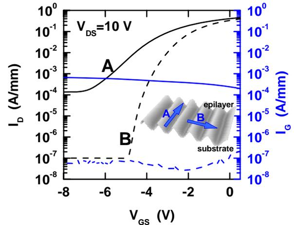
FIGURE 1. TRANSFER CHARACTERISTICS IN THE SATURATION REGIME FOR DEVICE A (SOLID LINE) AND DEVICE B (DASHED LINE) WITH  $L_G = 0.9\ \mu\text{m}$ ,  $L_{S-D} = 3.3\ \mu\text{m}$  AND  $W = 150\ \mu\text{m}$ . THE INSET ILLUSTRATES THE DIRECTION OF THE CURRENT WITH RESPECT TO THE POTENTIAL PROFILE INDUCED BY STEP EDGES.
