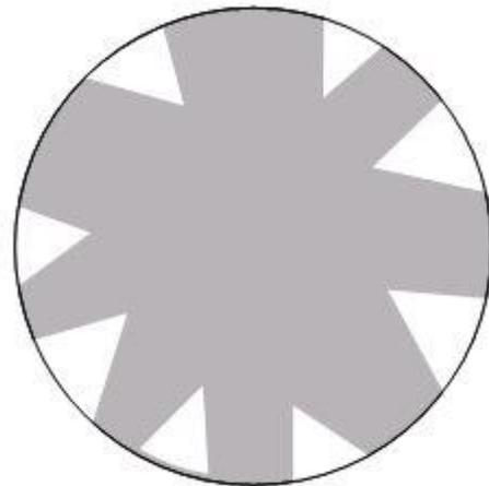
Figure 2 – Shark-Teeth Coating Defect
