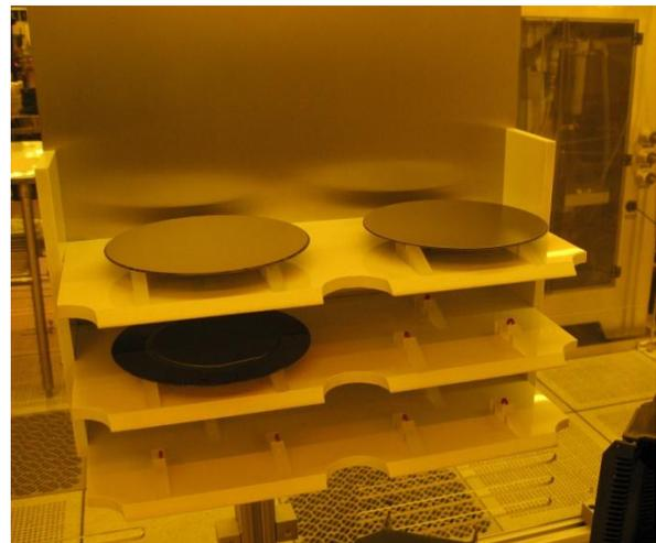
Figure 4 – Cooling Racks Inside Mount Tool
