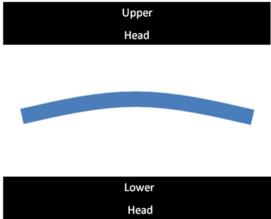
Figure 3. Exaggerated schematic of a bowed wafer between EC coils. The center is closer to the upper coil and so will register as a higher conductance and hence a lower sheet resistance.
