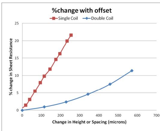
Figure 4. Influence of height difference on accuracy of double coil eddy current systems. We contrast with the single coil and see that the double coil has much less sensitivity to height differences.
