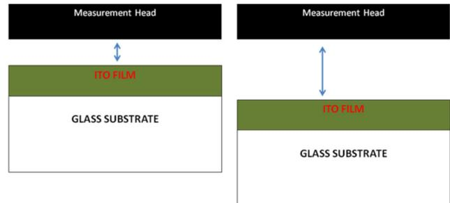
Figure 1. Example of two possible sample-head positions in a manual single coil EC system. A difference from probe-sample spacing compared to the calibration sample introduces error.
