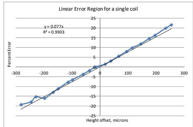
Figure 2. Influence of height difference on accuracy of single coil eddy current system. The error is 0.77% for each micron of height difference.
