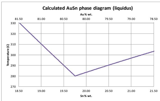
Fig. 3 AuSn phase diagram near the eutectic composition
