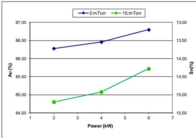
Fig. 5 Deposited AuSn composition as function of power
