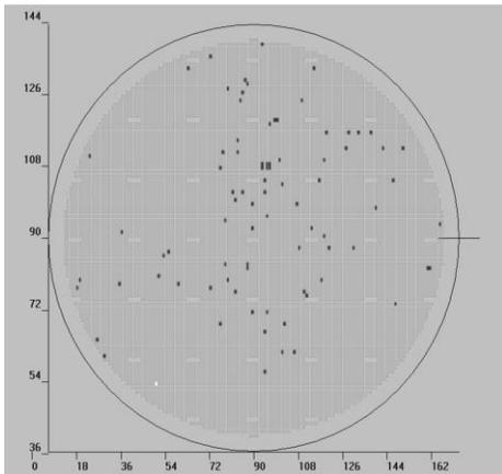
Figure 2. NSX-100 wafer map for the PV strip process with CoatsClean™ showing 99.3% die yield.
