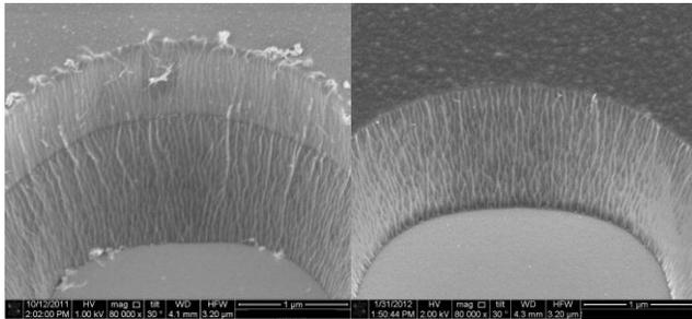
Figure 1. SEM images of the PV strip process: [left] unstripped showing photoresist (top layer) and polyimide (bottom layer), and [right] after the CoatsClean™ strip showing only the polyimide layer.
