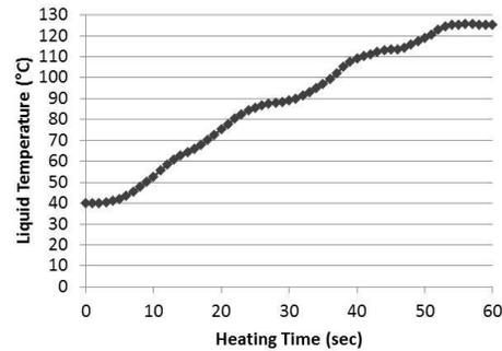
Figure 3. Liquid temperature vs. heating time for the BP strip process. The liquid temperature was measured by immersing a thermocouple bead in solution on a wafer in the EVG 301RS.
