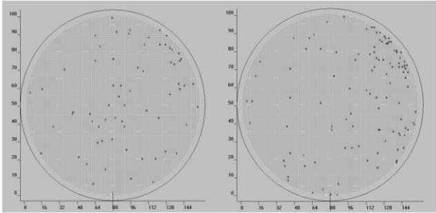
Figure 5. NSX-100 wafer maps for the BP strip on full-flow wafers: [left] CoatsClean™ processed wafer with 99.4% die yield and [right] standard Skyworks processed wafer with 99.1% die yield.
