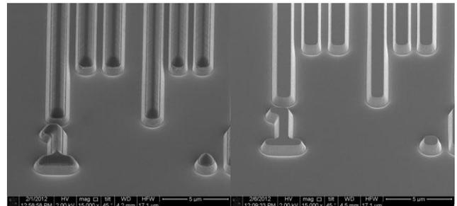
Figure 4. SEM images of the BP strip process: [left] unstripped and [right] after CoatsClean™ strip.
