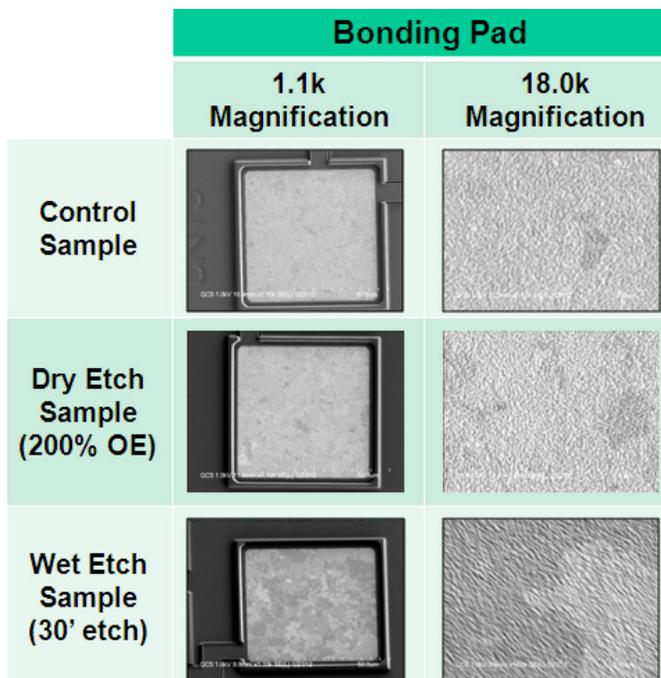
Figure 1: SEM image of bond pad area after TiO<sub>x</sub> removal.
