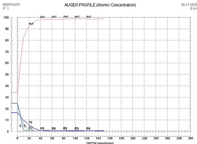
Figure 3: Auger depth profile of a dry etch sample with 100% over etch at via etch.
