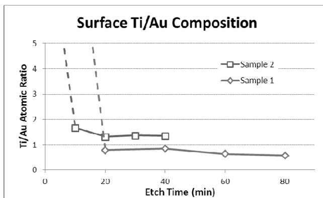
Figure 4: Surface Ti/Au Ratio of samples after wet etch
