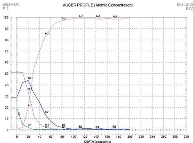
Figure 2: Auger depth profile of the control sample
