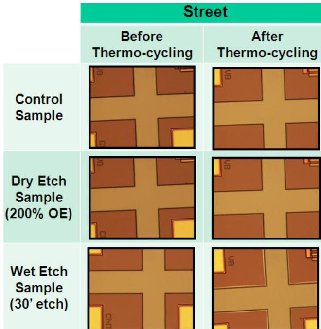
**Figure 5: Street area after thermal cycling for 10cycles at 260°C.**
