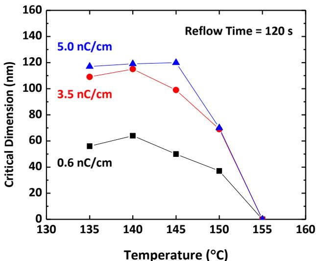
Figure 6 – ZEP feature size as a function of reflow temperature. The reflow duration was 2 min for all samples.
