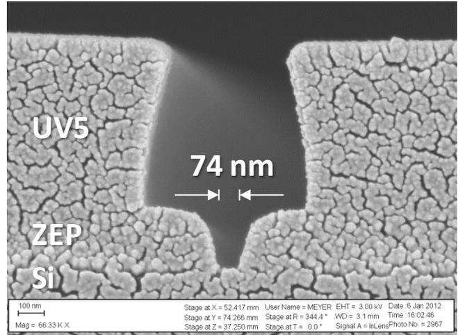
Figure 3 – Cross-section of UV5 feature on reflowed ZEP line (dose = 5.0 nC/cm, 10 min reflow at 145 °C). After development of UV5, a 20 sec  $\text{O}_2$  plasma descum was performed.
