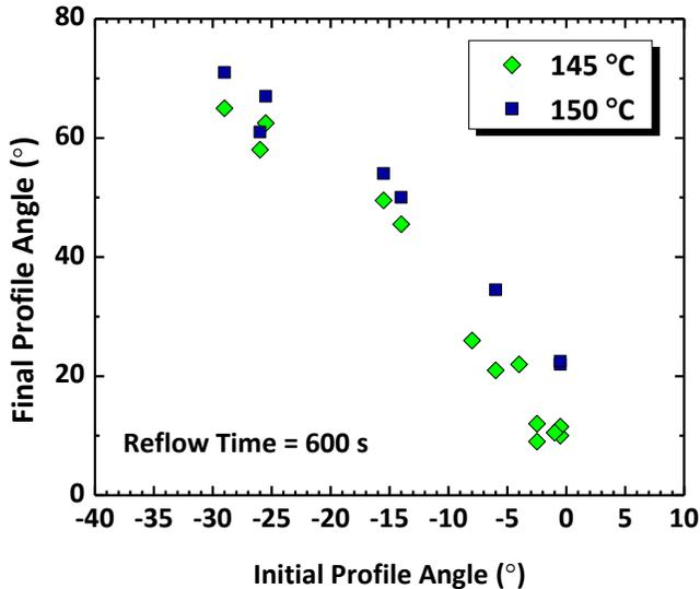
Figure 9 – ZEP feature final angle vs. initial angle for 10 min reflow at 145 °C or 150 °C.
