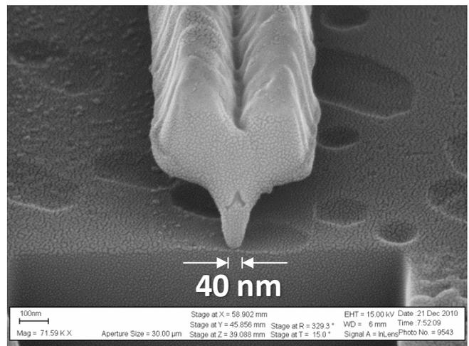
Figure 5 – FIB cross-section of 40 nm T-gate on AlGaIn/GaN mechanical wafer. The imaging angle is tilted 30° from the wafer surface.
