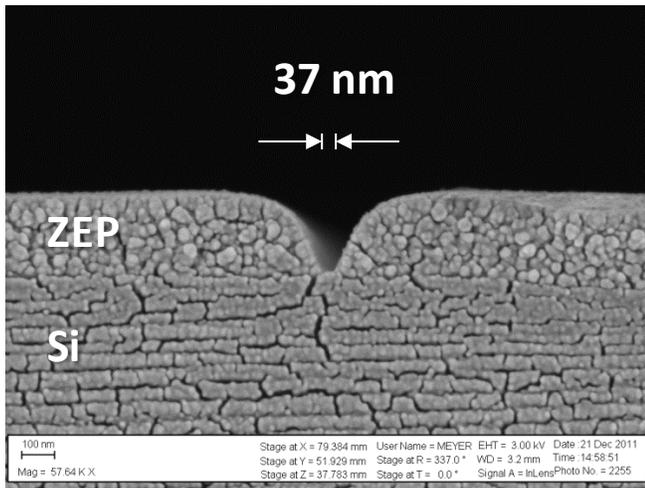
Figure 2 – Cross-section of ZEP line (dose = 5.0 nC/cm) after 10 min reflow at 145 °C.
