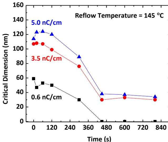
Figure 7 – ZEP feature size as a function of reflow time at 145  $^{\circ}\text{C}$ .
