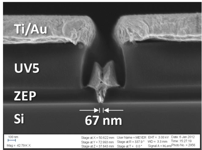
Figure 4 – Cross-section of metalized UV5/reflowed ZEP line (dose = 5.0 nC/cm, 10 min reflow at 145 °C, 20 s  $\text{O}_2$  plasma descum).
