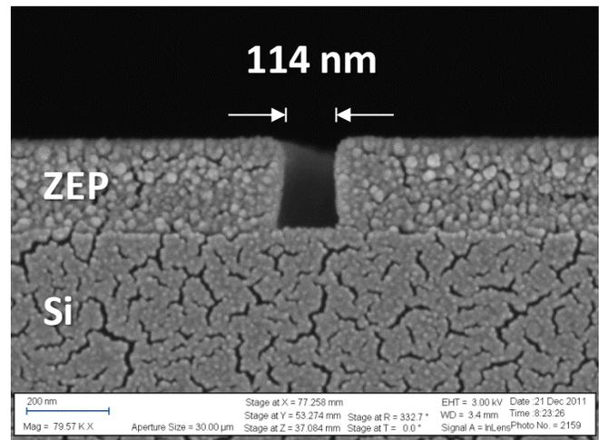
Figure 1 – Cross-section of as-developed ZEP line (dose = 5.0 nC/cm).
