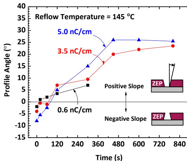
Figure 8 – ZEP feature angle as a function of reflow time at 145  $^{\circ}\text{C}$ .
