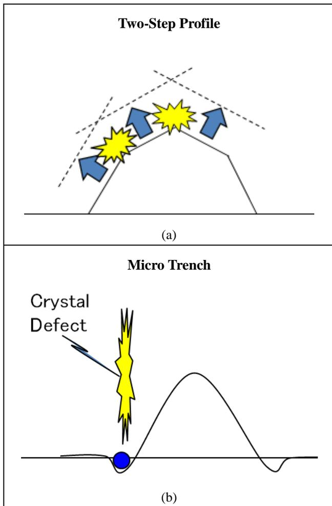
Figure 2. PSS shape and crystal defects. PSS profiles that produce epitaxial defects: (a) Two-step profile causes differences in the crystal growth direction, increasing the probability of imperfections around the top of the profile. (b) Micro-trenches on the fringe of the dot cause an “air gap” to form during crystal growth, increasing the probability of imperfections above the trench.
