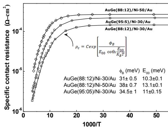
Figure 9. Specific contact resistance plotted as a function of inverse temperature for three AuGe alloy with different Ni layer thickness.
