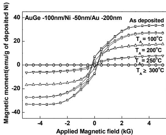
Figure 1. Magnetization loops for AuGe/Ni(50 nm)/Au annealed at various anneal temperatures.
