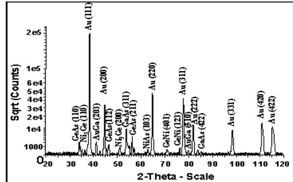
Figure 7. GIXRD measurements on AuGe/Ni (25nm)/Au annealed at 400°C and which shows the least contact resistance.
