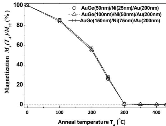
Figure 2. Anneal temperature dependence of saturation magnetization of contacts with same Ni/AuGe ratio.
