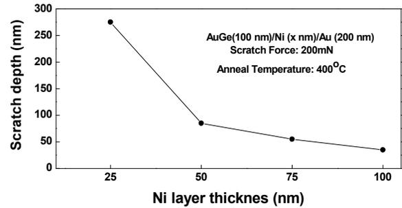
Figure 6. Scratch depth  $V_s$  Ni layer thickness.
