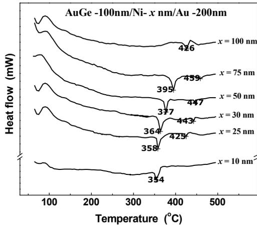
Figure 5. DSC scans for samples with eutectic AuGe alloy and different Ni layer thicknesses.
