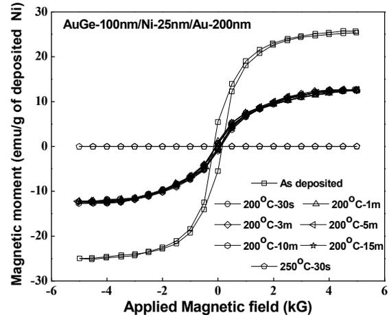
Figure 3. Magnetization as a function of anneal durations.
