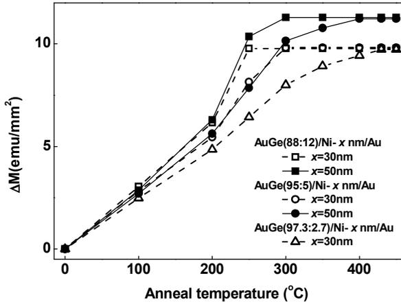
Figure 4. Effective thickness of Ni layer transformed to non-magnetic phase on annealing at various temperatures.
