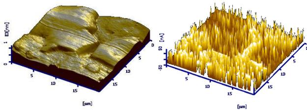
Figure 8. (a) Topography and (b) current image of an AuGe/Ni (30nm)/Au sample.
