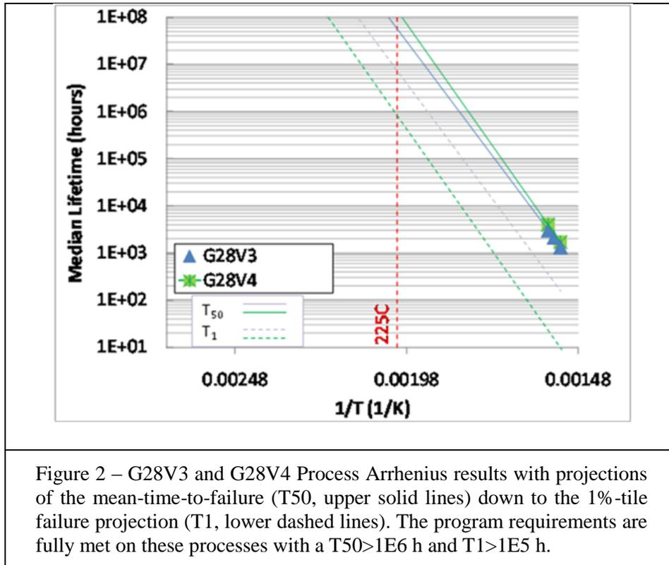
Figure 2 – G28V3 and G28V4 Process Arrhenius results with projections of the mean-time-to-failure (T<sub>50</sub>, upper solid lines) down to the 1%-tile failure projection (T<sub>1</sub>, lower dashed lines). The program requirements are fully met on these processes with a T<sub>50</sub>>1E6 h and T<sub>1</sub>>1E5 h.
