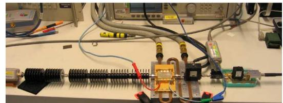
Fig.2 HPA module test bench for electrical characterization
