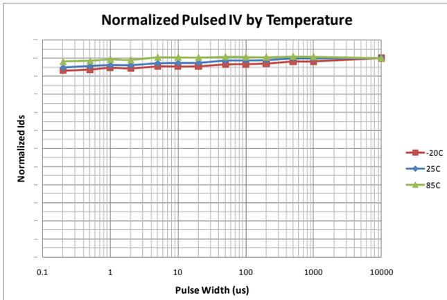
Figure6. Normalized pulsed IV response by temperature of present ultra fast switch speed FET at Vgs pulsed from -5V to 0.5V and Vds pulsed from 0 to 0.5V
