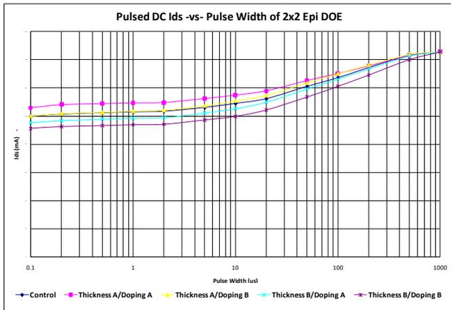
Figure2. Room temperature pulsed IV response of epi doping and epi thickness factors using high trap density fab process
