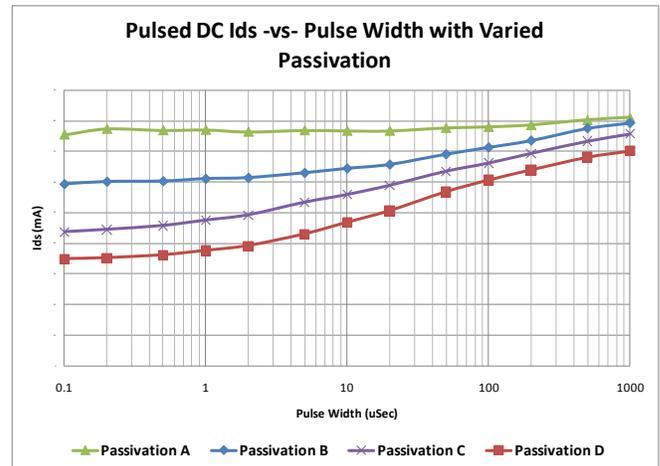
Figure5. Room temperature pulsed IV response of by passivation method using improved epi, and lower trap density fabrication processing
