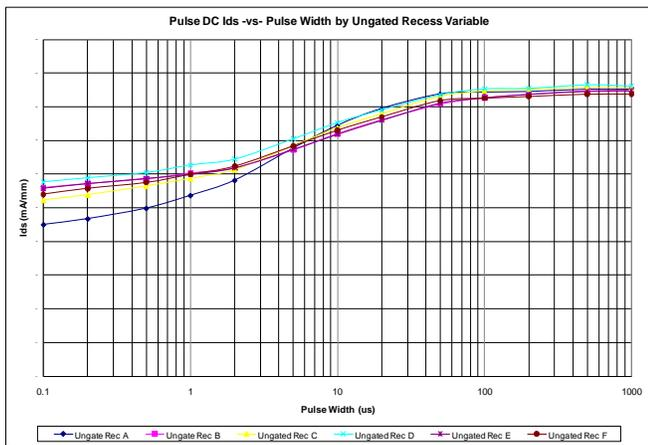
Figure3. Room temperature pulsed IV response of varied ungated recess conditions using high trap density fab process
