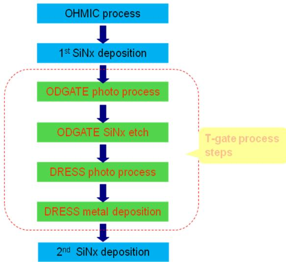
Fig.1 Overview of process sequence for transistor formation
