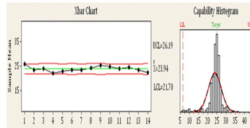
Fig.8 Wafer acceptance test capability of ft (GHz) (wafer basis)
