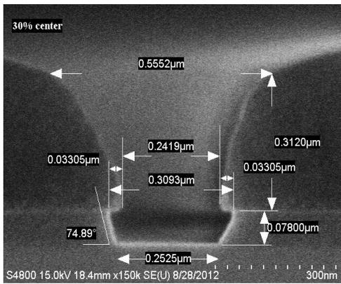
Fig.3 SiN sidewall profile after ODGATE patterning, after ICP etch, and with photoresist still present
