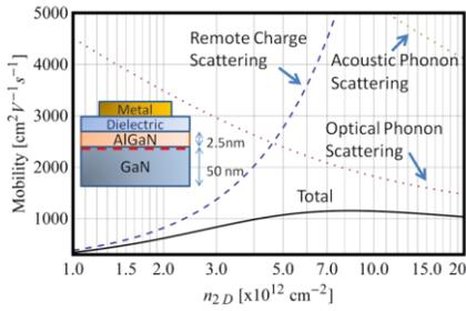
Fig.2. Simulation results – Mobility vs. 2DEG density.
