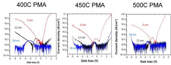
Fig.5. C-V profiles and flatband voltage for Al<sub>2</sub>O<sub>3</sub> on (a) (b) N-polar GaN and (c) (d) m-plane GaN with different PMA temperature.
