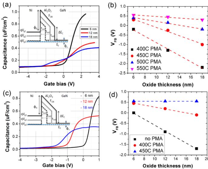
Fig.7. C-V profiles for 15nm Al<sub>2</sub>O<sub>3</sub> / 19nm Al<sub>0.3</sub>Ga<sub>0.7</sub>N / GaN MISHEMT with different PMA temperature.
