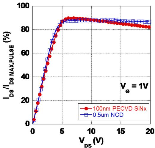
Figure 3. Current collapse in NCD-capped and SiNx-passivated HEMTs under DC operating conditions, quantified by decrease in  $I_{DS,MAX}$  relative to pulsed I-V.
