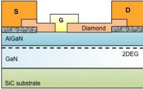
Figure 1. Schematic of “Diamond after Gate” HEMT with diamond directly On GaN
