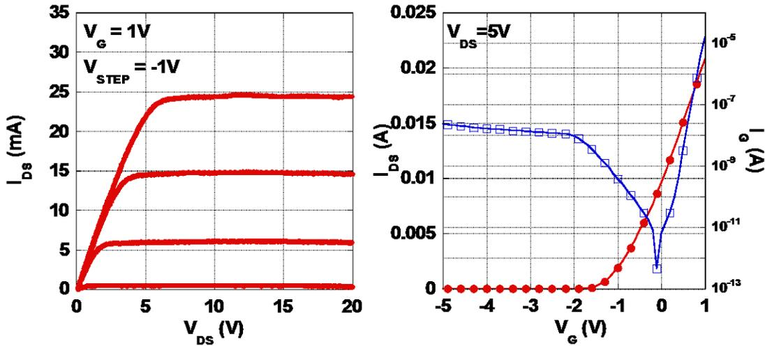
Figure 2. Transfer curves for NCD-capped HEMT with diamond directly on GaN
