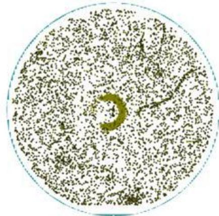
Figure 1: Horn Defect
