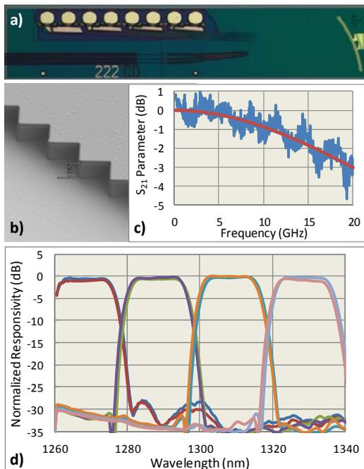
**Figure 4.** 4x25G CWDM receiver PIC for 100Gb/s FOI. a) – the optical microscope image of as-fabricated chip after die singulation; b) – the SEM image of the etched DEG; c) – the frequency response of the PIN-WPD; d) – normalized fiber-coupled responsivity spectra in TE / TM polarizations.
