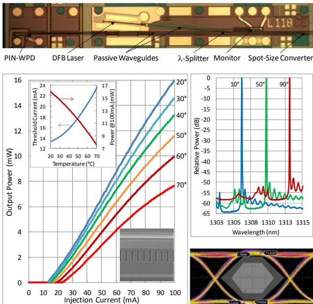
**Figure 2.** Full optical duplex PIC for ONU transceiver applications in FTTH networks. Top – optical microscope image of a 0.4mm x 2.8mm die after singulation; bottom – key performance features of the on-chip DFB laser. Shown in the bottom right corner of the light-current characteristic is the SEM image of the laser's vertically-coupled surface-etched grating.
