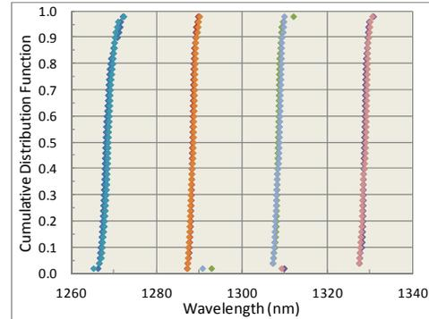
**Figure 5.** Cumulative distribution functions for the centre wavelengths of the DEG-based 4-channel CWDM filter at 25C. Total of 265 integrated receiver chips from different wafers / lots tested in both TE and TM polarizations. Average inter-channel spacing is 20.08nm (target: 20nm).
