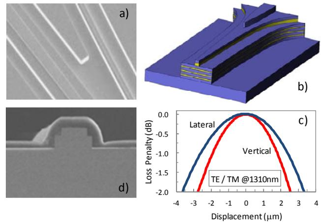
**Figure 1.** On-chip SSC – the most generic MGVI building block. a) and d) – the top view and vertical cross-section SEM images, respectively; b) – sketch of the SSC featuring multiple-step lateral tapering; c) – measured insertion loss penalty vs. displacement from the optimal alignment position.
