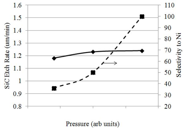
Figure 6 SiC via etch rate and mask selectivity vs pressure. SF<sub>6</sub>/O<sub>2</sub>/He flow rate ratio 10:1:25.
