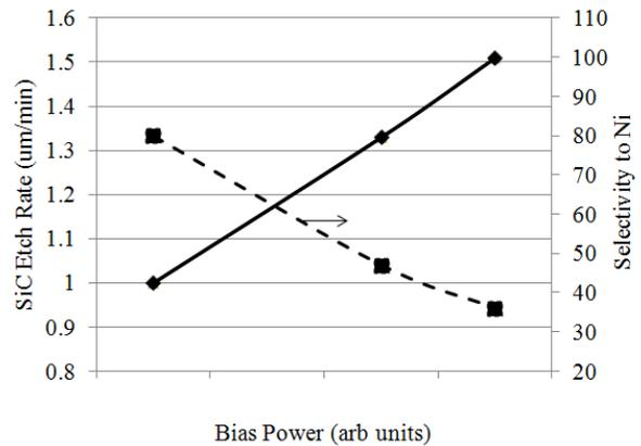
Figure 3 SiC via etch rate and mask selectivity vs bias power. SF<sub>6</sub>/O<sub>2</sub>/He flow rate ratio 10:1:7.
