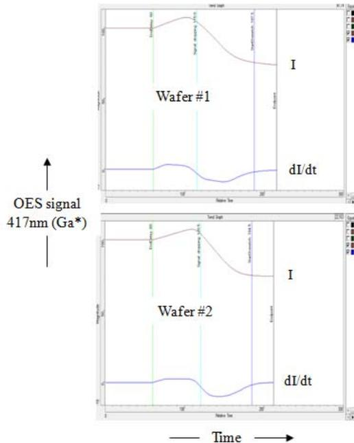
Figure 9 OES end-point traces for 2 consecutive GaN etches stopping on Au.
