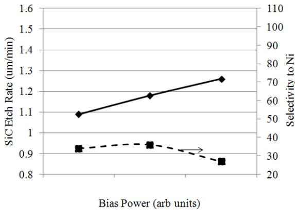
Figure 5 SiC via etch rate and mask selectivity vs bias power. SF<sub>6</sub>/O<sub>2</sub>/He flow rate ratio 10:1:25.
