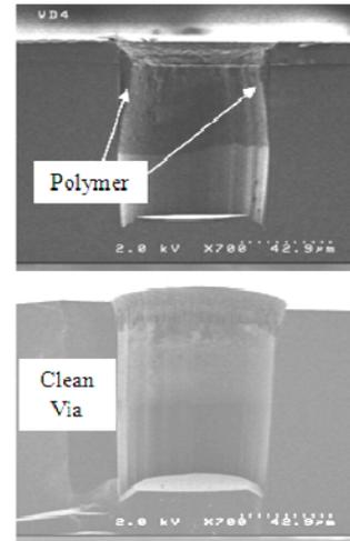
Figure 10 Partial via etches before and after polymer removal in 20% HNO<sub>3</sub> 15 minutes.
