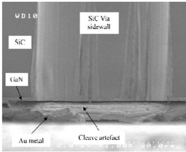
Figure 8 Base of SiC via after GaN etching.
