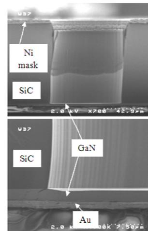
Figure 7 100µm deep SiC via etched to the GaN layer. GaN loss measured at <0.35µm.
