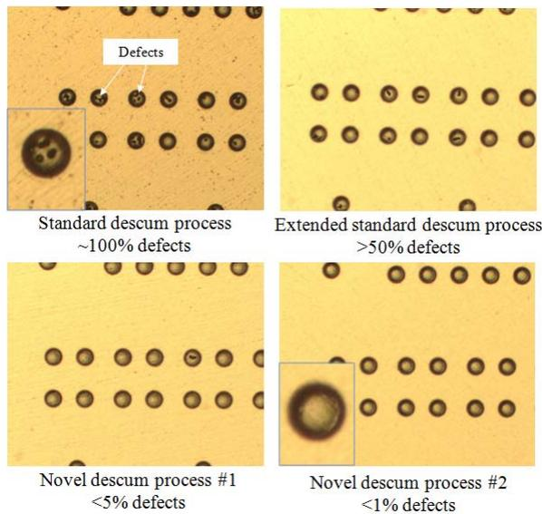
Figure 2 Optical images showing the effect of descum conditions on pillar defect density.
