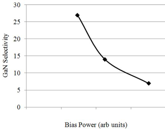
Figure 4 SiC:GaN selectivity ratio vs bias power. SF<sub>6</sub>/O<sub>2</sub>/He flow rate ratio 10:1:7.
