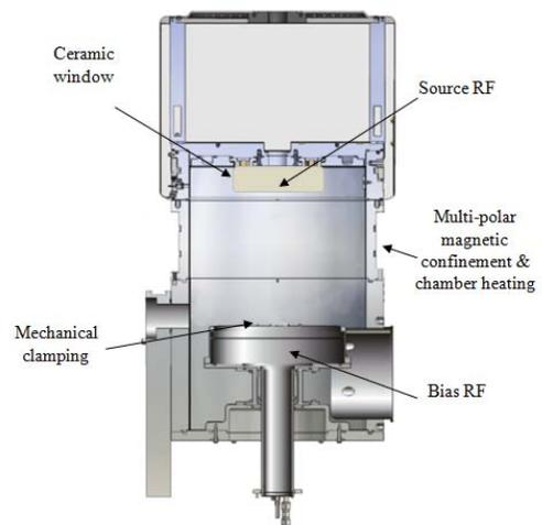
Figure 1 Schematic diagram of the APS plasma etch module.
