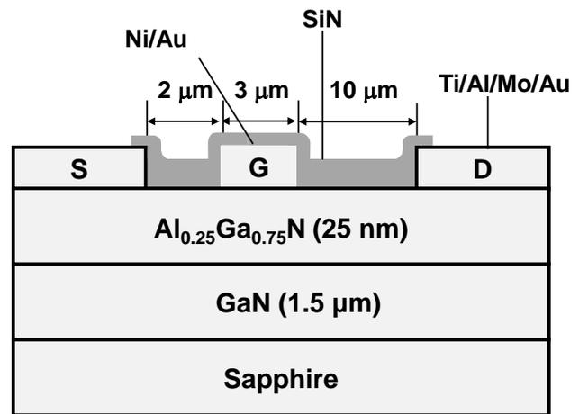
Fig.1 Schematic cross-sectional structure of  $\text{Al}_{0.25}\text{Ga}_{0.75}\text{N}/\text{GaN}$  HEMT on sapphire substrate.
