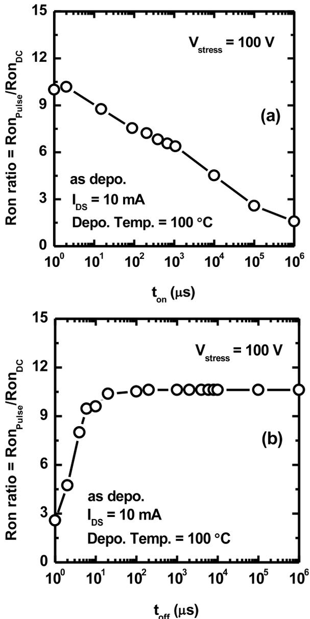
Fig. 5  $R_{ON}$  ratio transients for device A. On-state time (a) and off-state time (b). At on-state time dependent measurement,  $t_{off}$  was fixed 1 ms and off-state time,  $t_{on}$  was fixed 1  $\mu s$ .
