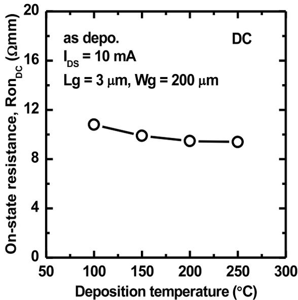
Fig. 2 On-state resistance,  $R_{ON(DC)}$  vs. deposition temperature.
