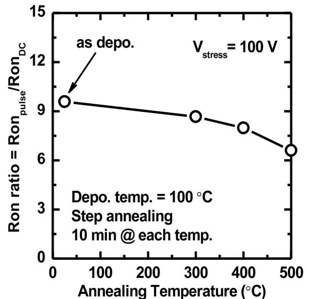
Fig. 4  $R_{ON}$  ratio vs. annealing temperature.
