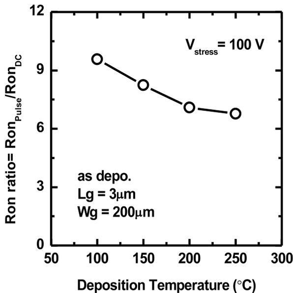
Fig. 3  $R_{ON}$  ratio as a function of deposition temperature.
