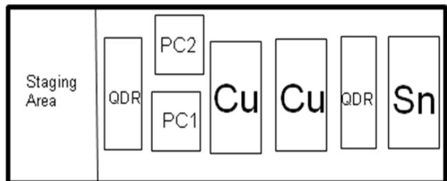
**Figure 2. Plating Sink Configuration.**
