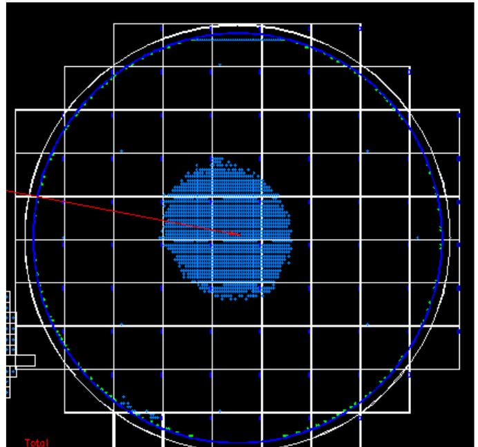
**Figure 6: 3D AOI Wafermap showing defects on the center of the wafer**
