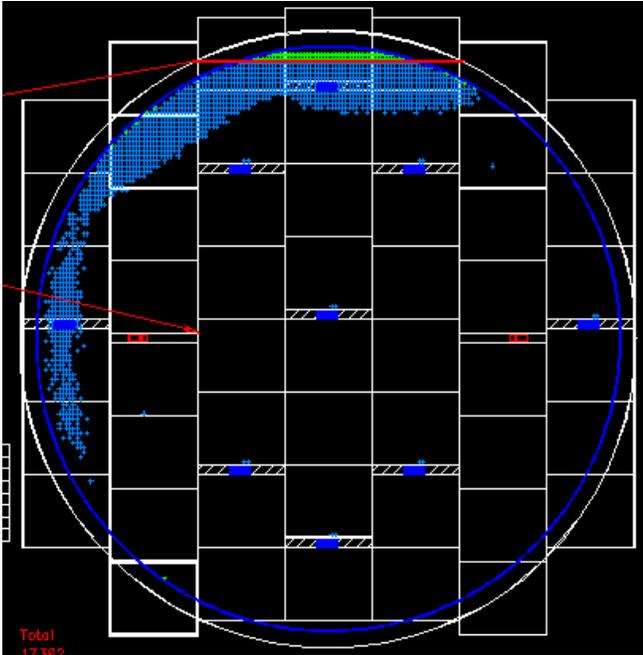
**Figure 7: 3D AOI wafermap showing defects on the edge of the wafer**
