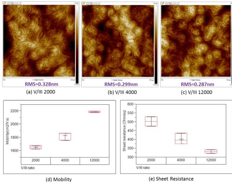
Figure 1: 5 $\mu\text{m}$  x 5 $\mu\text{m}$  AFM images and electrical properties of AlGaIn/GaN heterostructures with different V/III ratio (2000, 4000, 12000) at 920 °C with N<sub>2</sub>
