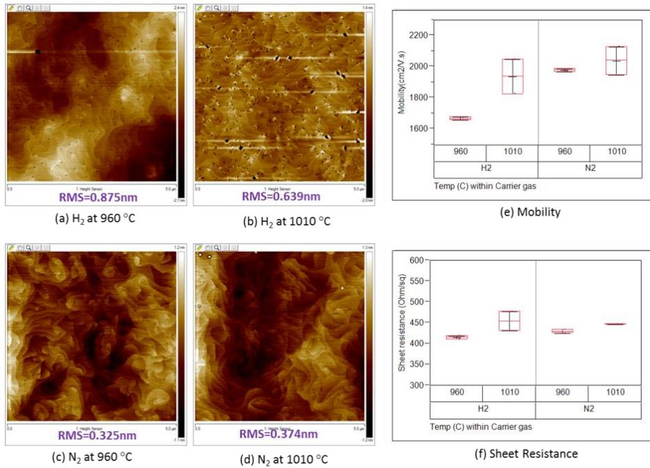
Figure 2: 5 $\mu\text{m}$  x 5 $\mu\text{m}$  AFM images and electrical properties of AlGaIn/GaN heterostructures with different carrier gas (H<sub>2</sub>, N<sub>2</sub>) and growth temperature (960 °C, 1010 °C)
