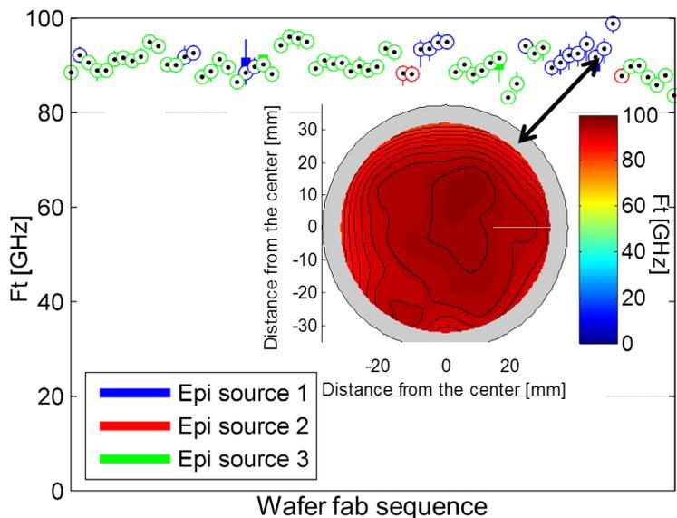
Figure 1: A trend chart box plot of Ft showing statistical box plots. Each column represents a wafer's statistical distribution. Solid boxes cover 25% to 75% of the distribution, and black dots indicate the median. The thin lines cover approximately 99.3% of the data distribution. Most
