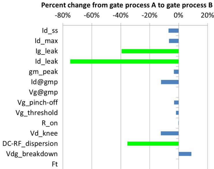
Figure 2: A bar chart comparing the percentage change of key performance parameters from the original gate process (A) to the new gate process (B). Green bars highlight significant changes. Only leakage currents and DC-RF dispersion were significantly affected by the processing change, and they were all improved.
