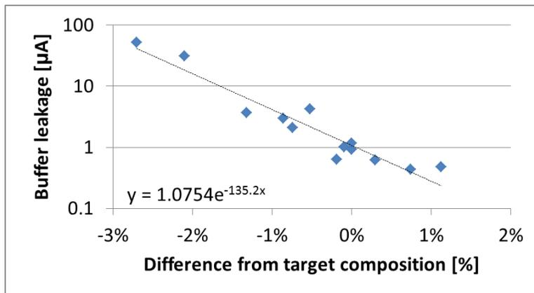
Figure 3: Correlation between wafer buffer leakage current and the difference from target epitaxial material composition, showing a strong relationship and fit with an exponential equation. This data was used to improve epitaxial material specification limits.
